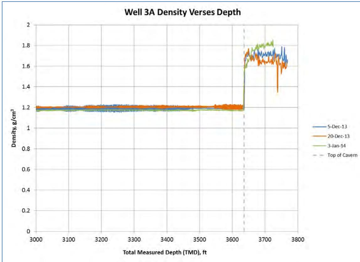
**Figure PRAL.** Recent Density versus Depth Logs from Well 3A. Logs indicate a sharp density increase at the top of the Oxy-3 cavern (3636 ft TMD).
