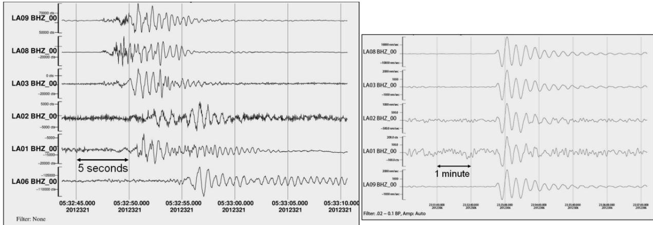
Figure 3 . Examples of seismic signals recorded at Grand Bayou USGS seismic array broadband stations (vertical component). Left plot is an example of a high frequency “MEQ” seismic signal (recorded 16 November 2012 at 5:32 UTC). Right figure is a VLP seismic signal (recorded on November 3, 2012, at 23:35 UTC). Records are from the USGS surface seismic array (see Figure 1 for station locations).
