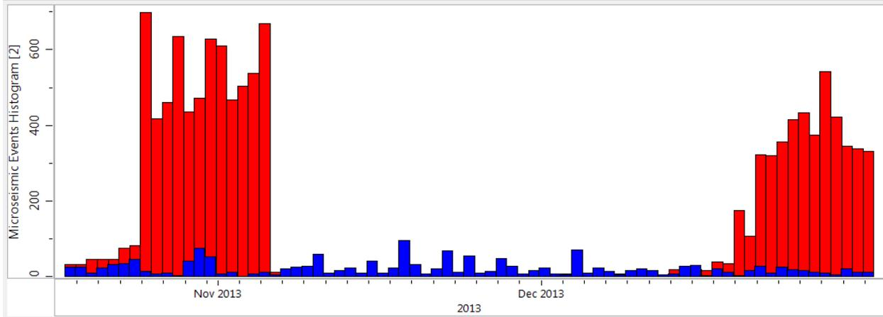
Figure 6. Histogram of the number of shallow (<1000 ft) MEQ (red) and deep (>1000 ft) MEQ (blue) detections per day from 18 October to 31 December 2013 reported by MAGNITUDE from G-01 borehole seismic array.
