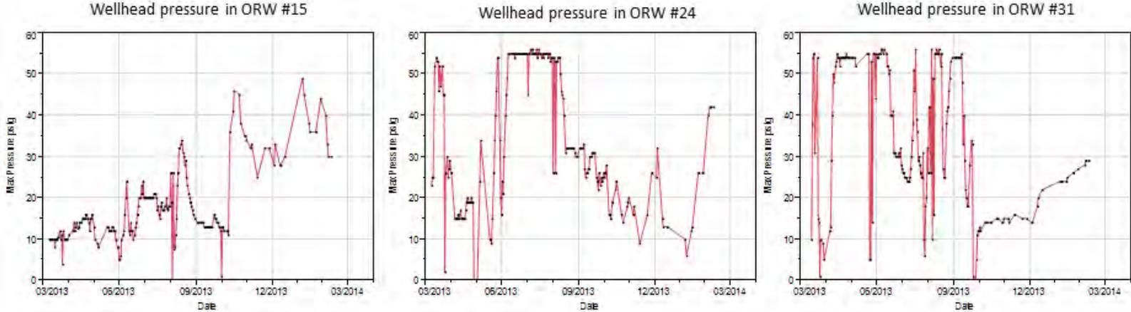
Figure 3. Wellhead pressures from selected wells on Dugas-LeBlanc property. Data from LDNR daily checklists.
