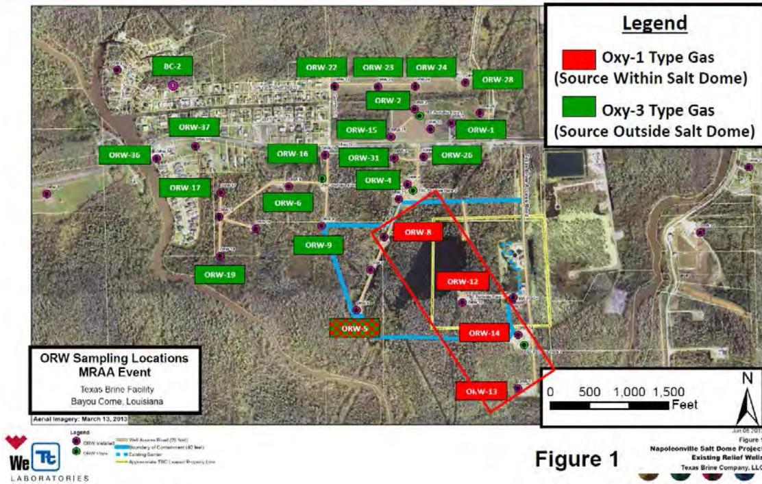
Figure 1. The gas venting from the MRAA at ORWs primary consists of Oxy-3 type thermal gas northwest of the sinkhole, and Oxy-1 type thermal gas between the sinkhole and the Napoleonville salt dome.
