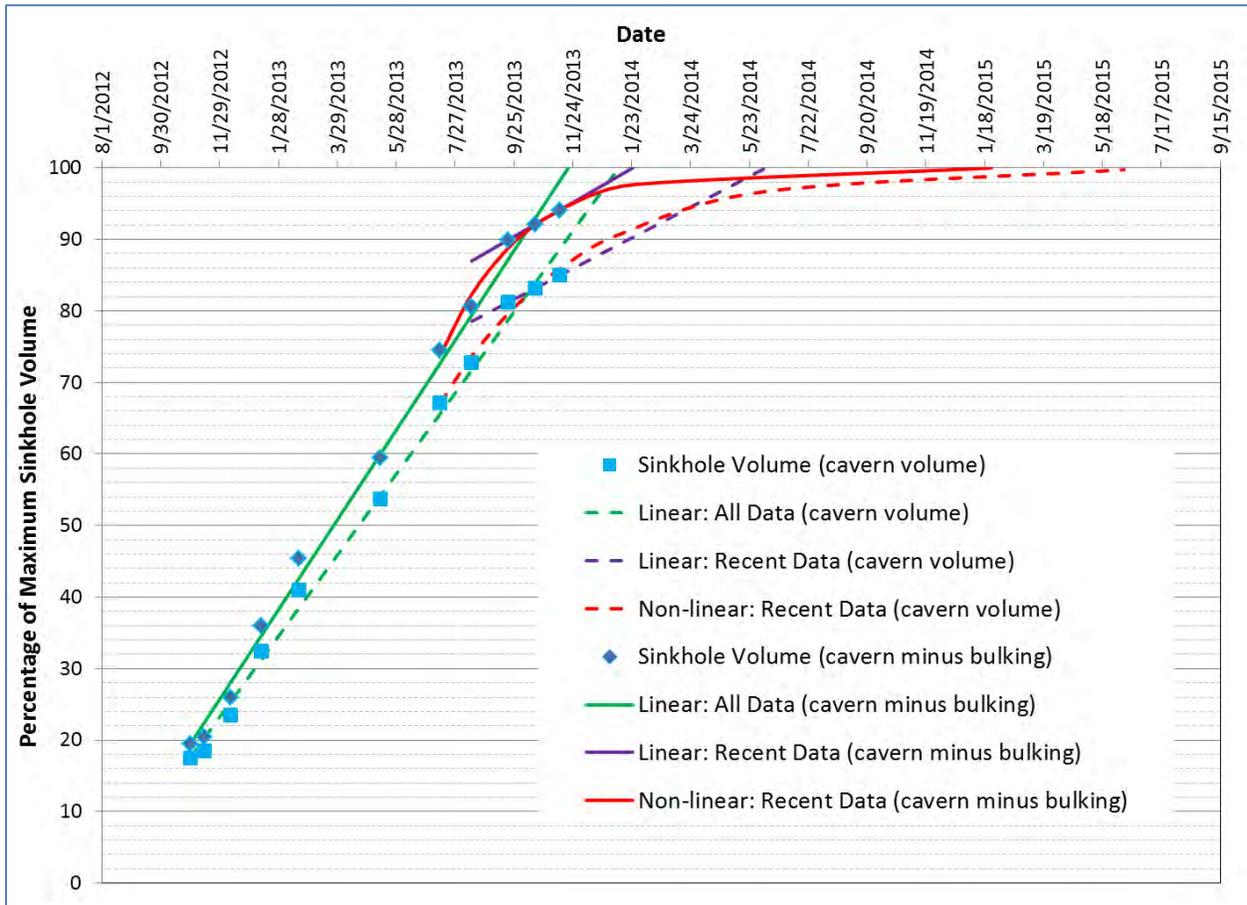
**Figure LineFit.** Temporal Trend of Sinkhole Volume based on Various Regression Techniques
