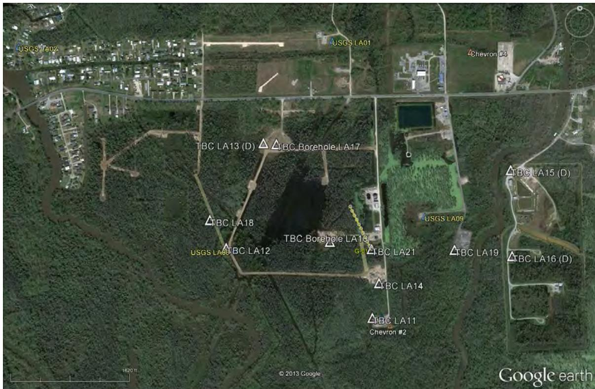
Figure 1. Google earth image of Grand Bayou area, the triangles indicate the station locations of the USGS, ESG and TBC seismic arrays, as labeled (not shown is ESG 8 is located in Bayou Corne, 2.5 mile west of the OG1 cavern). The letter “D” indicates a decommissioned Texas Brine station. The aerial Google Earth image shows the sinkhole geometry on 12 March 2012. Table 1 in the Appendix contains additional details on the seismic stations.
