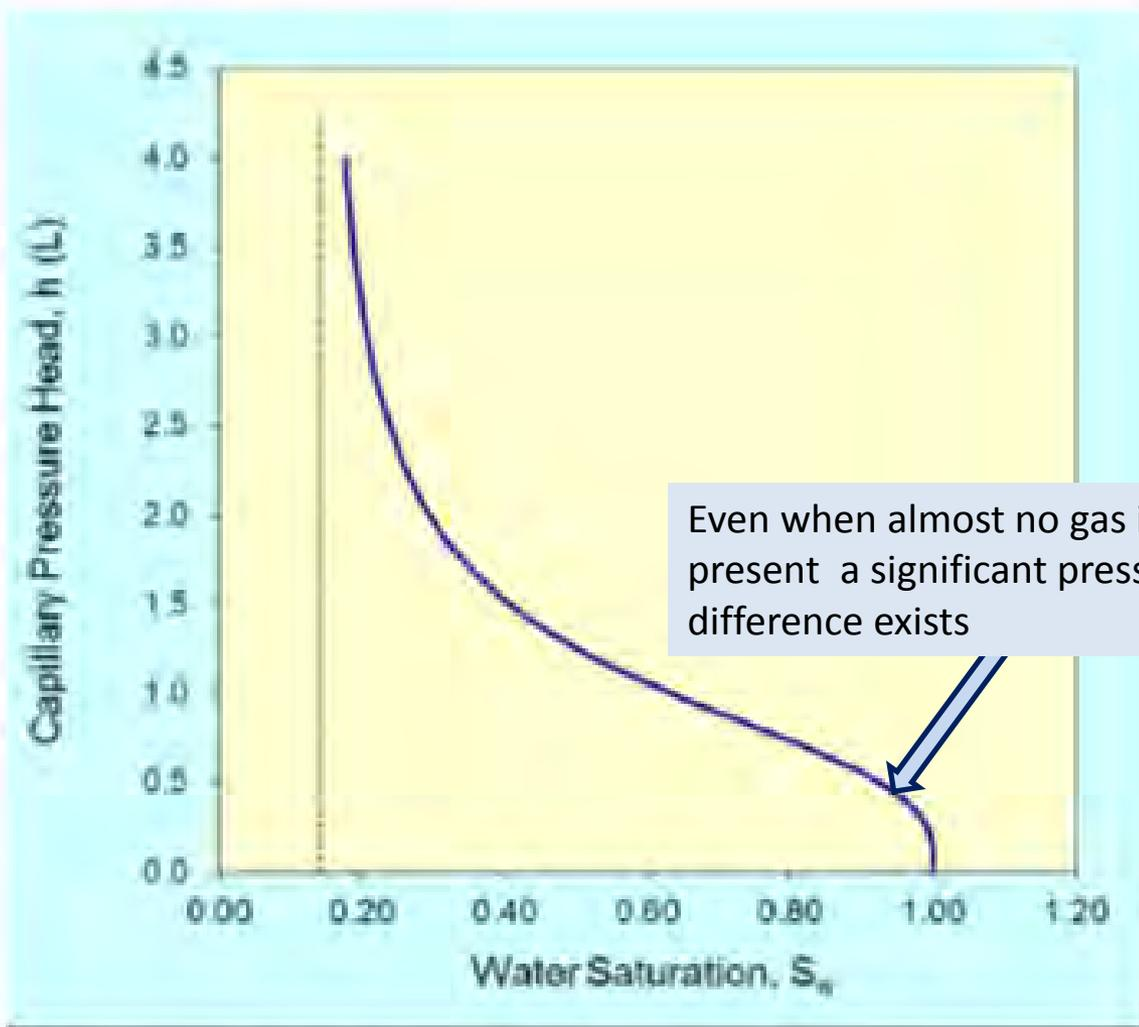
Figure 2. Representative soil characteristic curve for sand texture soil
