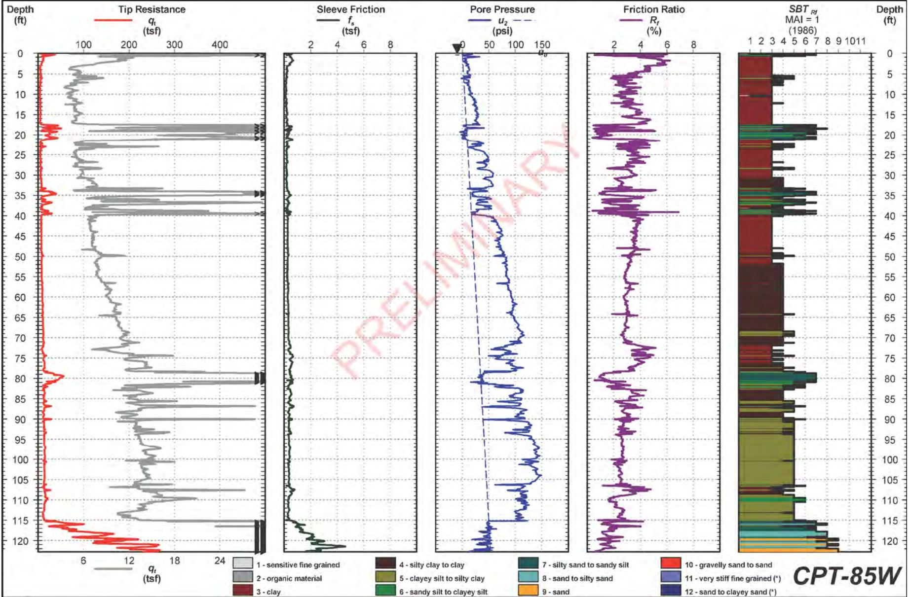
Figure 2. Summary plot of CPT-85 cone penetration test, near ORW-42.
