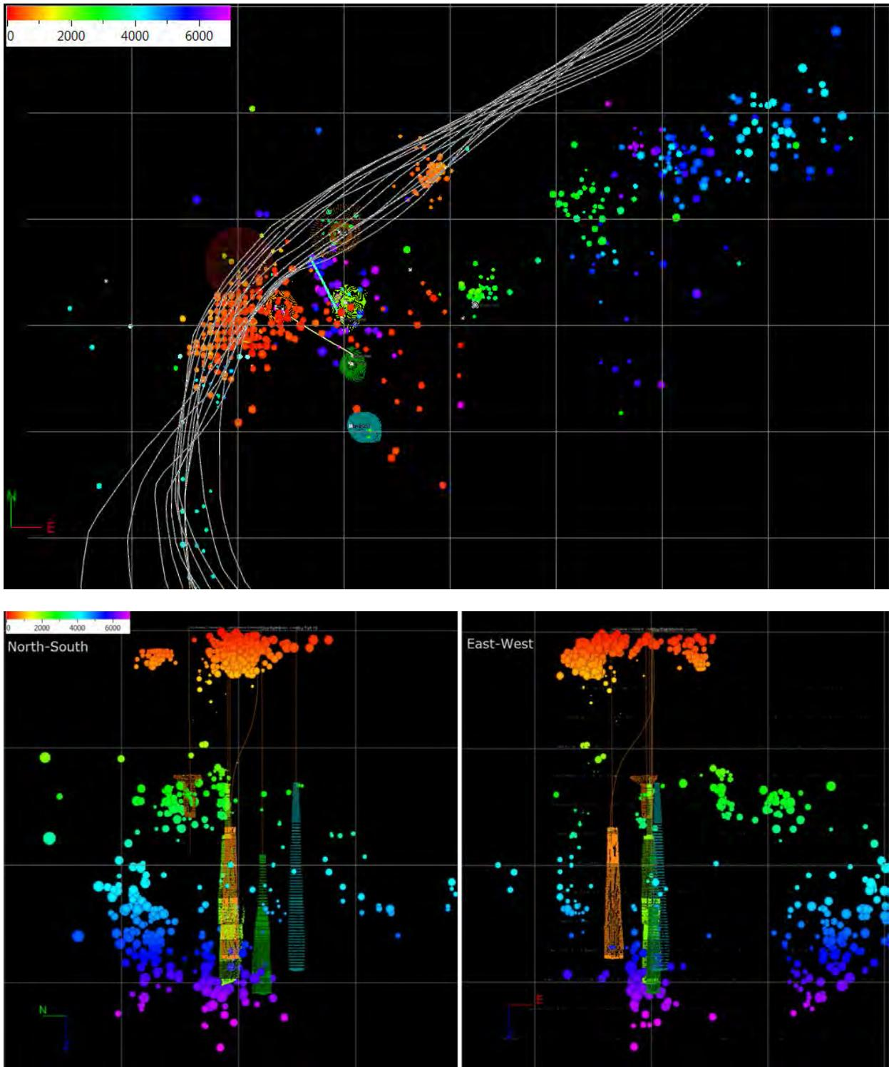
Figure 8. Map view, upper plot and cross sections (north-south section on the left and east-west section on the right with salt picks from 3D shown with dark gray dots) of MEQ events reported by MAGNITUDE with G-01 array with TBC cavern outlines. MEQ events colored by depth and sized by magnitude. Grid lines are 2000 feet. White contours in map view are the Napoleonville salt dome edge of salt picks from the 3D seismic >1000 ft.
