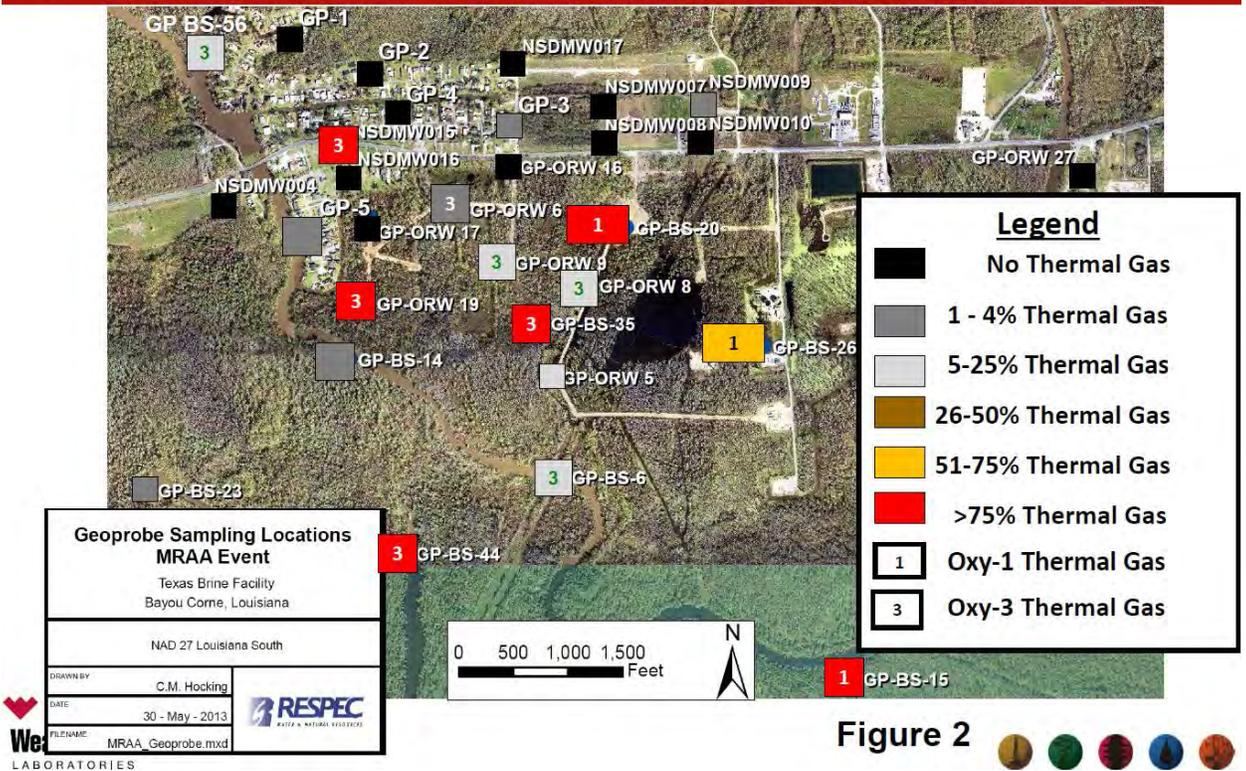
Figure 2. The amount of thermal gas dissolved in the MRAA aquitard varies widely, probably because thermal gas cannot migrate efficiently between laterally-discontinuous sand beds.
