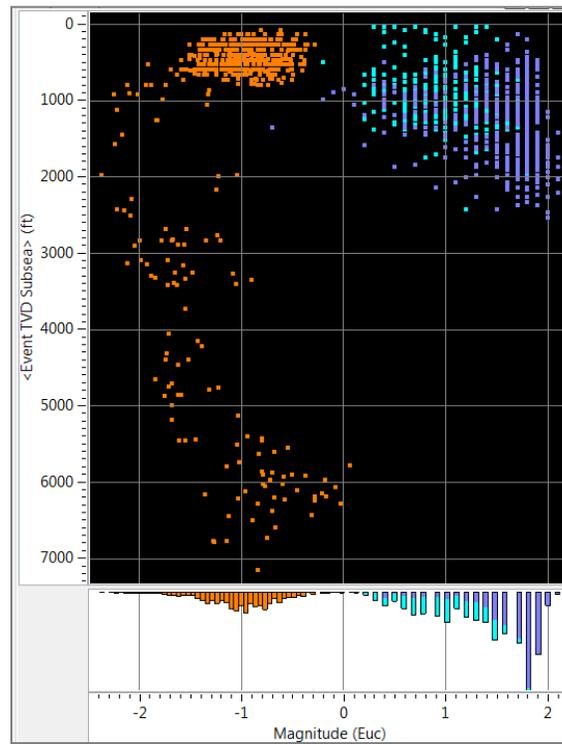
Figure 11. Comparison of MEQ depth and magnitude estimates using G-01 borehole array (orange) and CERI provided locations (TBC array data indicated by cyan dots, USGS array purple dots) depth and magnitude. Lower plot is a magnitude histogram comparison of the data sets.
