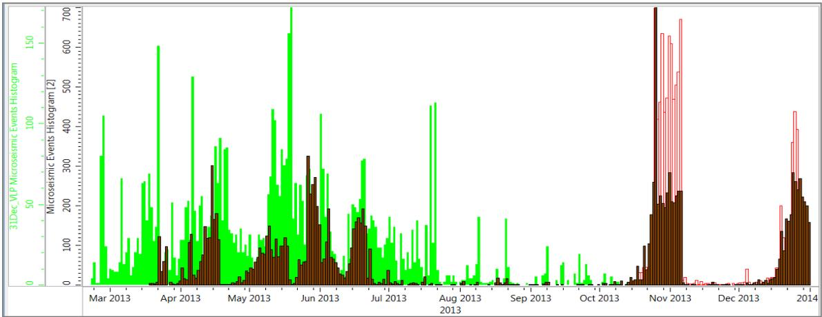
Figure 14. Histogram of MEQ and VLP detections from March-December 2013. Brown is MEQ counts from Nanometrics using the surface array. Green indicates VLP counts from Nanometrics. Red indicates shallow detections from G-01 array.
