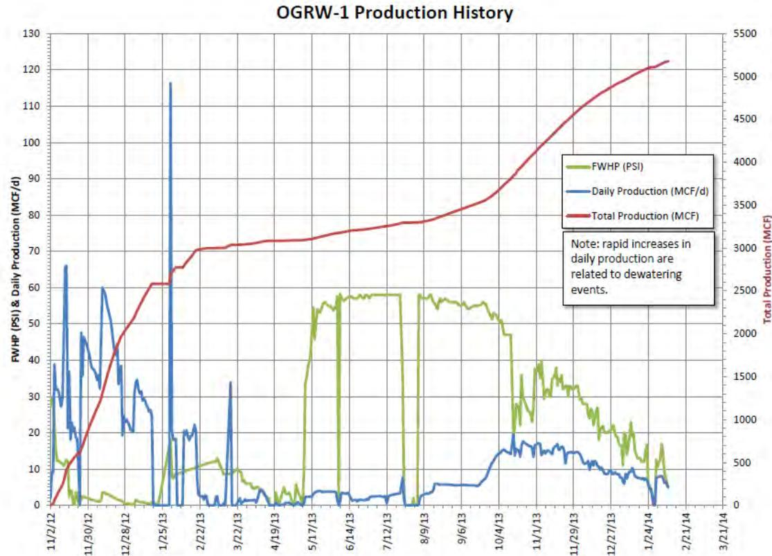
Figure 2. OGRW-01 flow pressure graph showing periods of high flow following well dewatering. Since August 2013, OGRW-01 has been continuously dewatered with a permanent pump.
