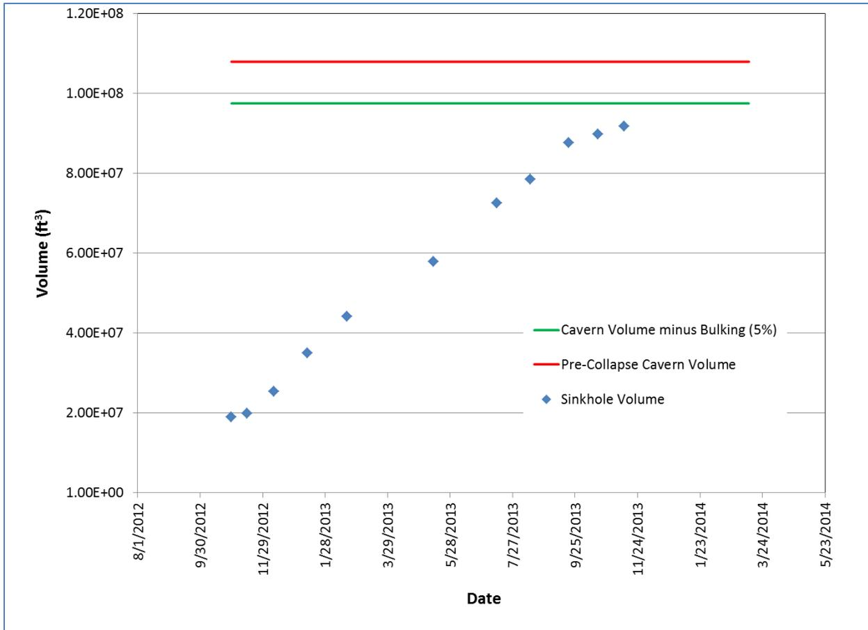
**Figure Volume.** Temporal Trend of Sinkhole Volume Shown Approaching Pre-collapse Cavern Volume.
