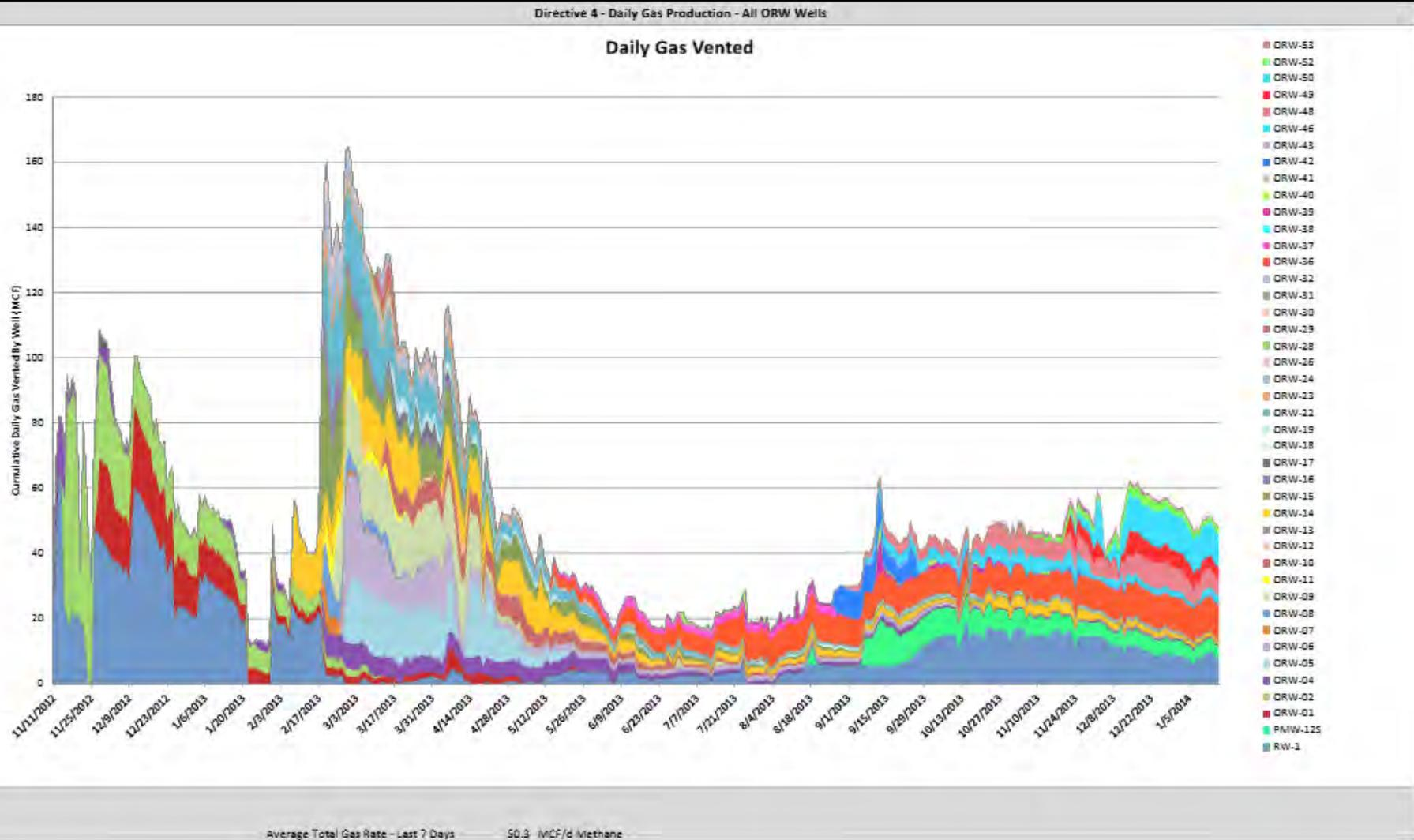
15 out of 47 wells venting and 6 wells account for 86.5% of gas vented (as of 17 JAN 2014)
