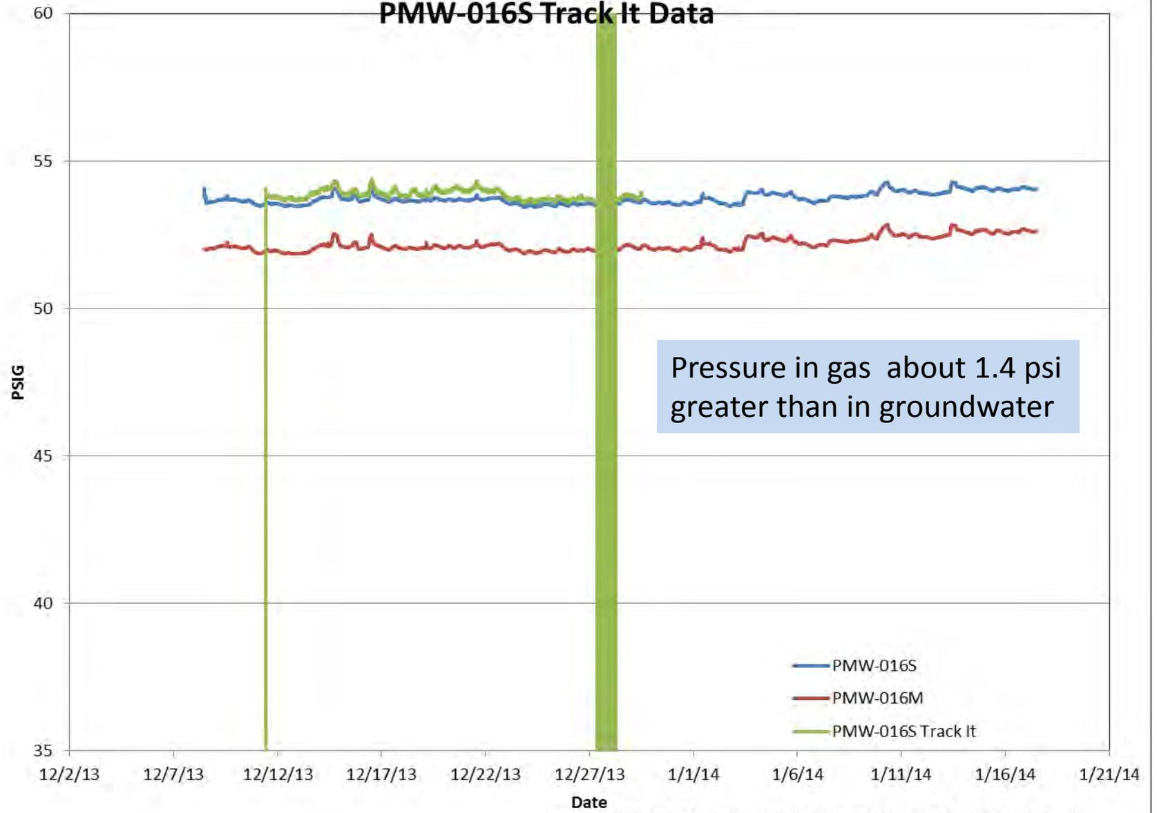
Pressure in gas about 1.4 psi greater than in groundwater
