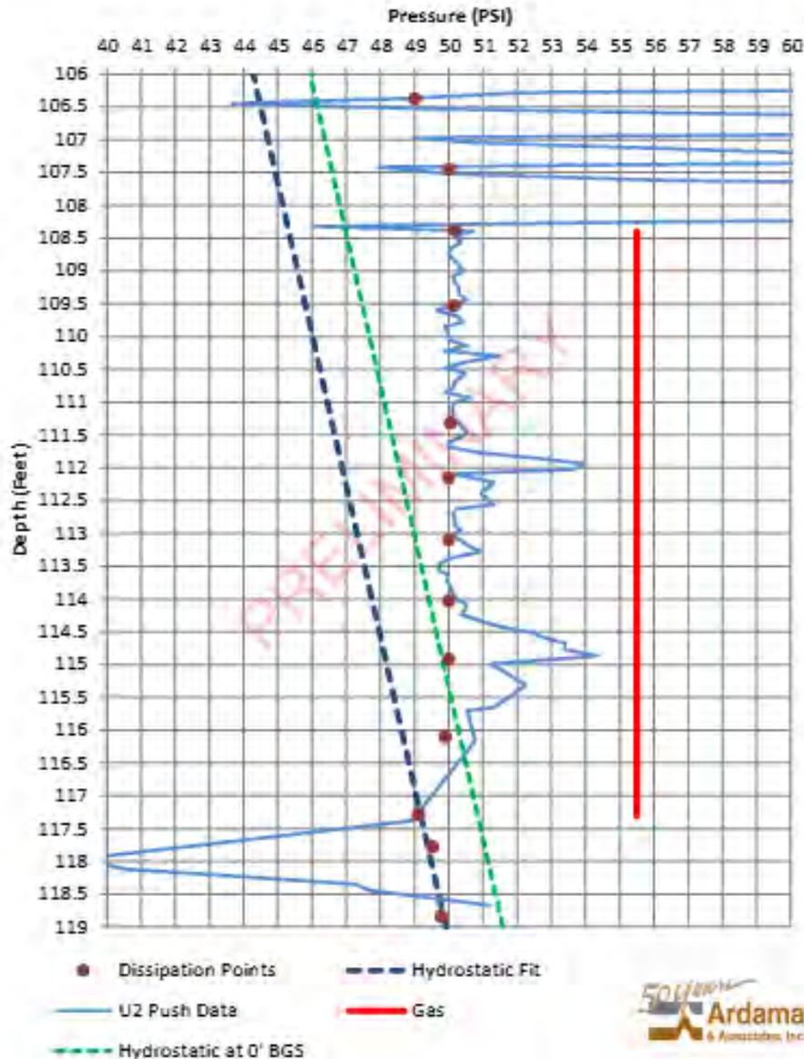
Gas cap pressure profile with hydrostatic pressure gradient below gas cap
