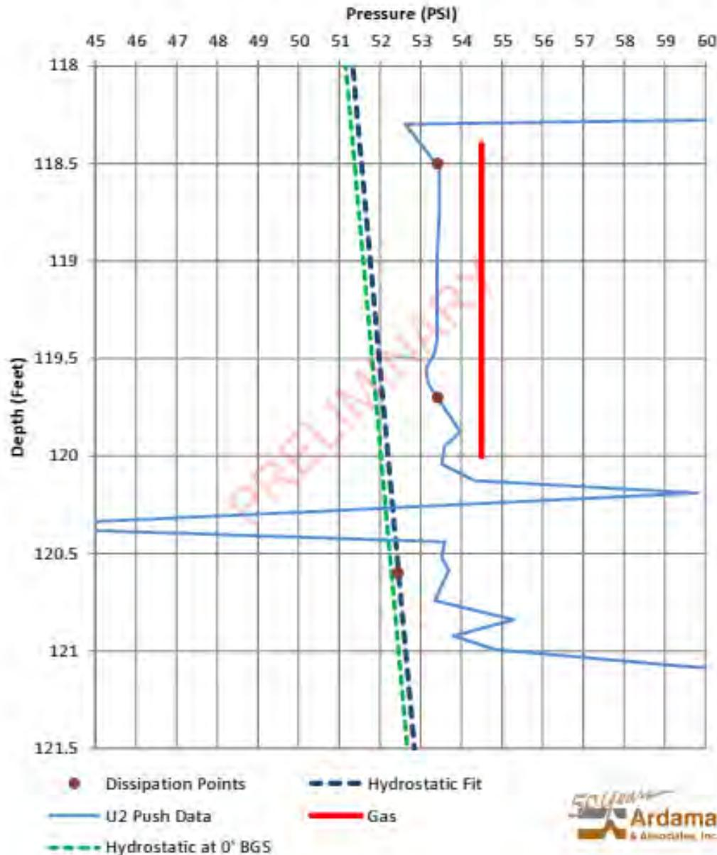
Gas and groundwater pressures greater than ground surface based hydrostatic pressures
