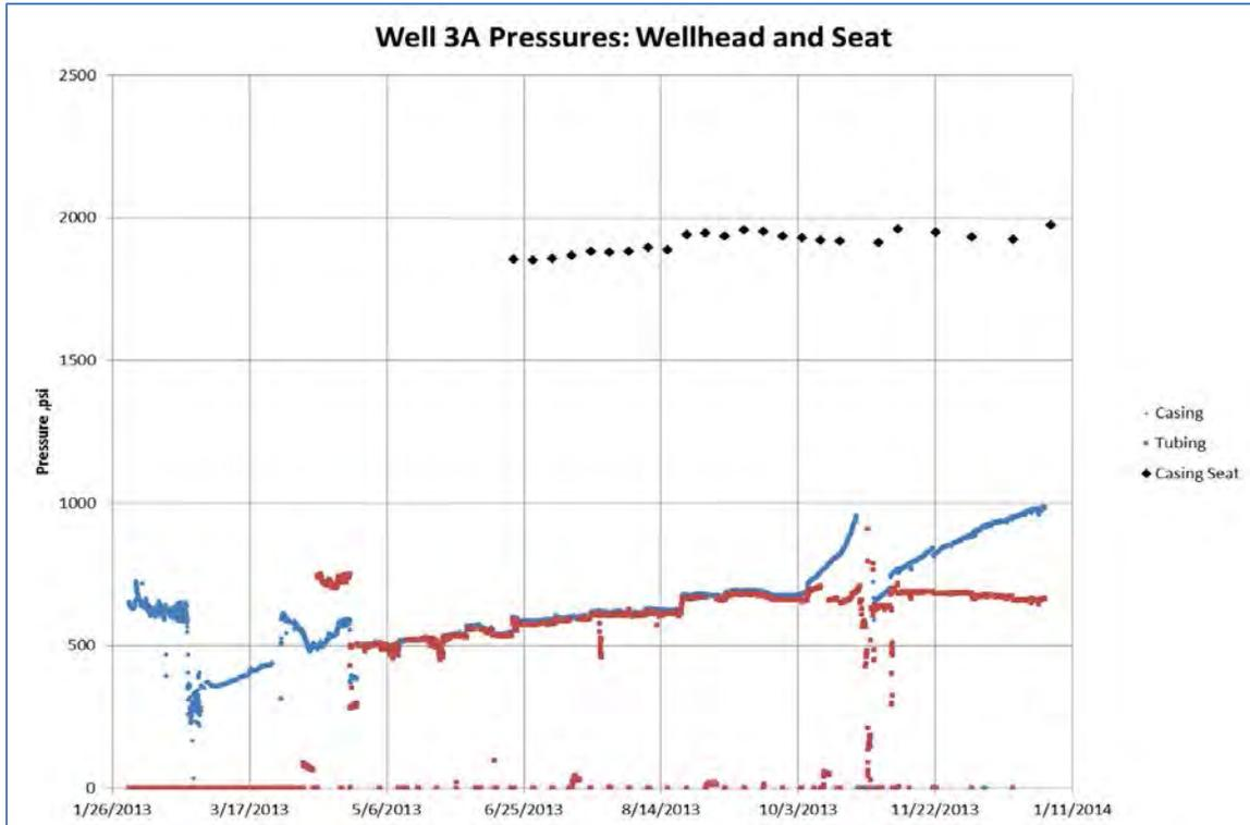
**Figure Pressure.** Casing and Tubing Pressure Measured at Wellhead 3A, and Borehole Pressure Measured at Casing Seat (2660' TMD).
