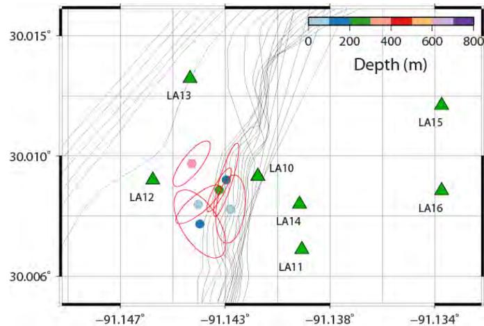
Figure 16. Event locations and depths for trigger events of hybrid VLP events computed by Weston Geophysical. Event uncertainty is indicated by ellipse surrounding each event. Gray lines mark the approximate salt boundary as mapped by vintage 3D seismic data. Green triangles mark the seismic stations used to compute the event location.
