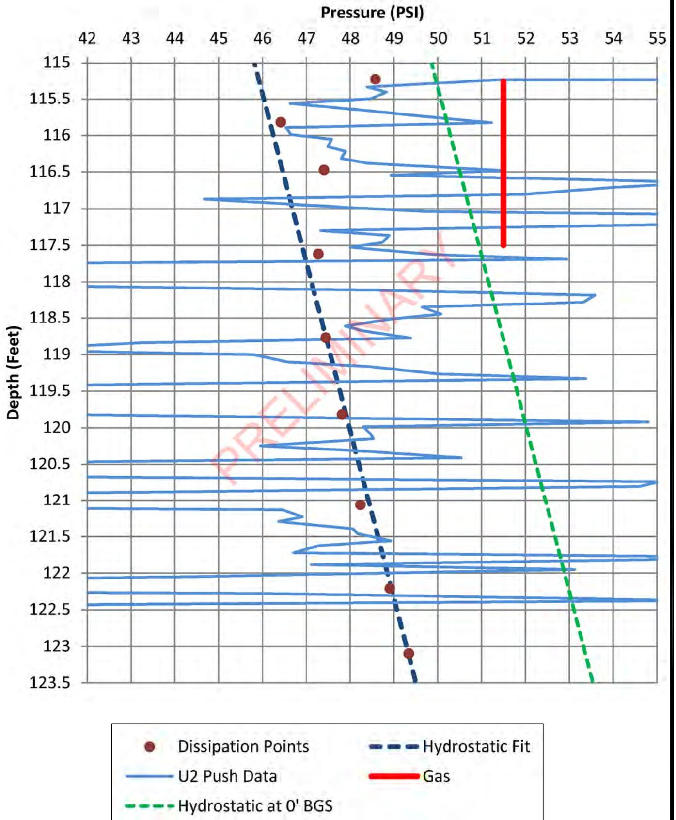
Figure 3. Dissipation points and interpretation of gas at top of MRAA for CPT-85W, near ORW-42.
