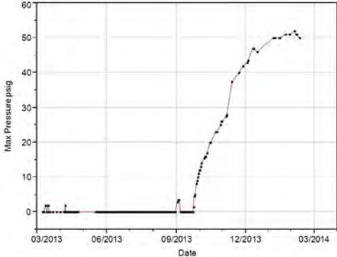
Figure 4. Time-series wellhead pressure data from pressure monitoring well TBC-03.
