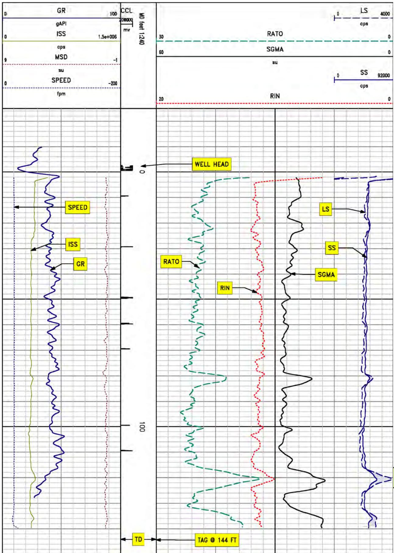
Figure 1. PDK log for ORW-42 showing inferred gas interval at top of MRAA.
