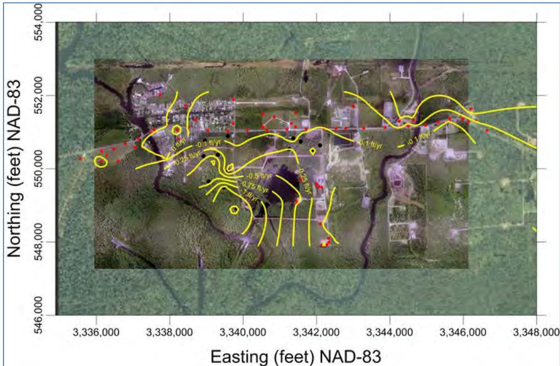
**Figure Contours.** Subsidence Rate Contours in Feet per Year Based on Fenstermaker Surveys and Water-Level Gauges [Van Sambeek, 2013b].
