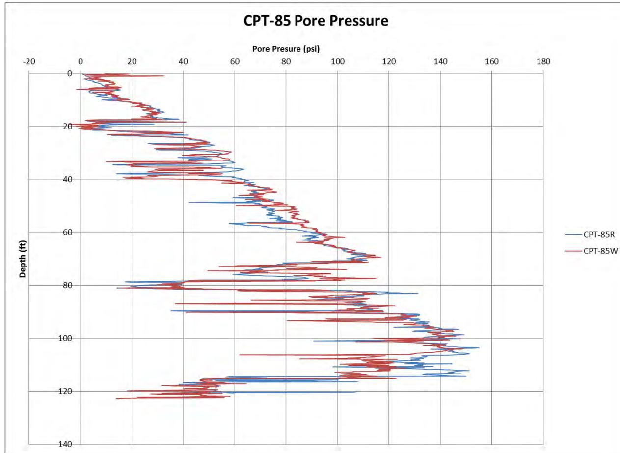
Figure 5. Repeat CPT pore pressure data curves.
