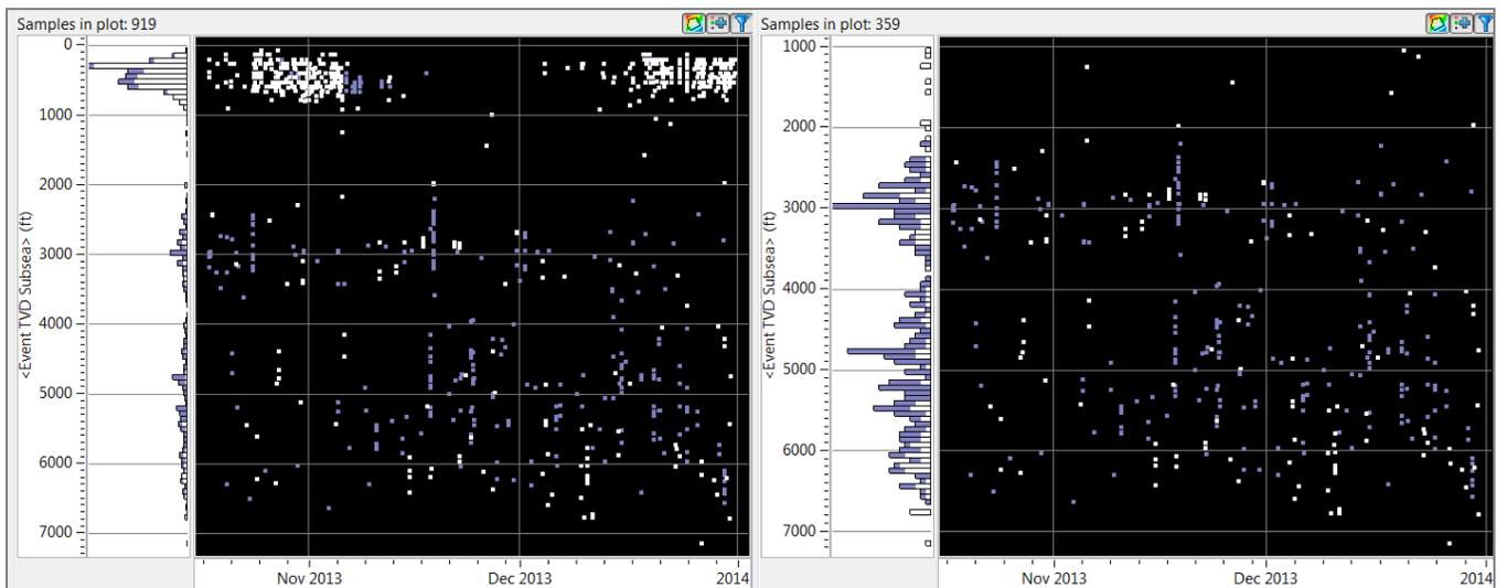
Figure 9. Time versus depth for all MEQ's located by G-01 array. White dots/histograms indicate events occurring within the TBC target zone defined by LDNR. Left plot shows all depth ranges, right plot, only events below 1000 feet to show detail of the microseismicity >1000 feet depth.
