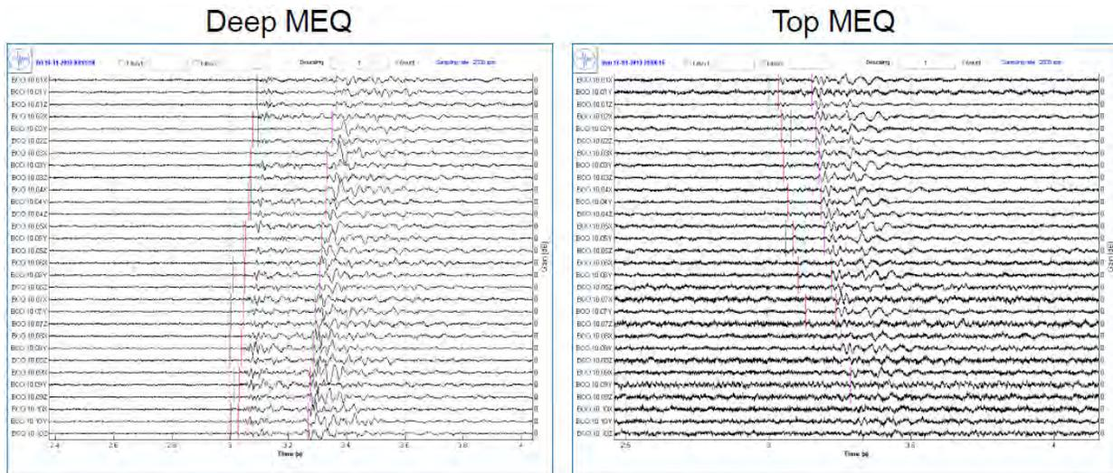
Figure 5. Seismic waveforms (time x axis and depth of geophone, top array show on top of the plot) recorded on the G-01 array showing examples of microseismic events detected below the array (left) and above the array (right). The direction of the energy, the “move-out” of seismic energy recorded on the borehole array was used to classify MEQ detections above and below the array.
