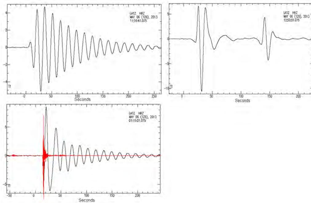
Figure 15. Examples of VLP recorded on broadband station LA12. Upper left, a “Classic” VLP with impulsive onset and exponential resonance decay, upper right, two VLP events with impulsive onset but no trailing resonance. Lower left figure is a “Hybrid” VLP-MEQ event, the red waveform is unfiltered data showing high frequency MEQ “trigger” event at onset of VLP, the VLP shown by filtered black waveform and the amplitudes have been normalized.
