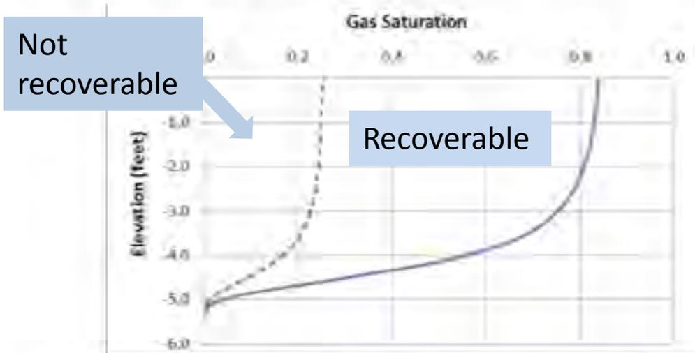
Figure 3. Calculated gas cap saturation distribution based on a gas pressure = 50 psig
