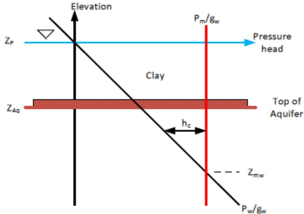
Figure 1: Pressure distribution for water ( $P_w$ ) and methane ( $P_m$ ) at the gas cap located adjacent to the top of aquifer
