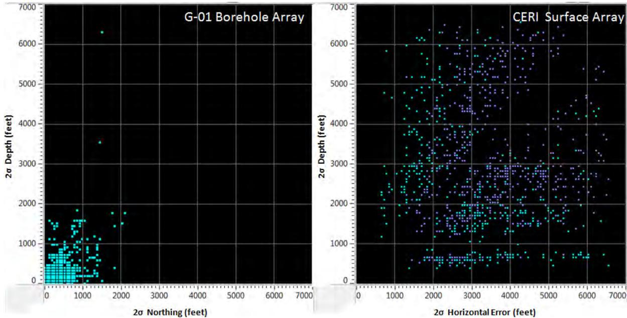
Figure 12. Comparison of estimated MEQ  $2\sigma$  location uncertainties in depth and horizontal position from G-01 array (left) and CERI surface locations of USGS (purple) and TBC (cyan) surface array. Graphs are scaled the same for comparison purposes. The uncertainties represent 2 standard deviations.
