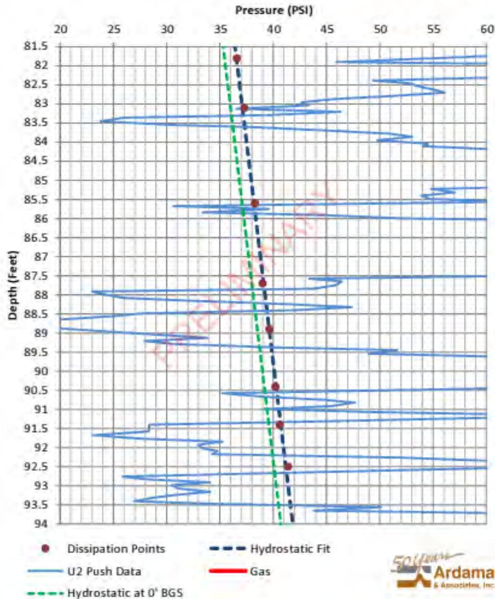
Groundwater pressures less than ground surface based hydrostatic pressures
