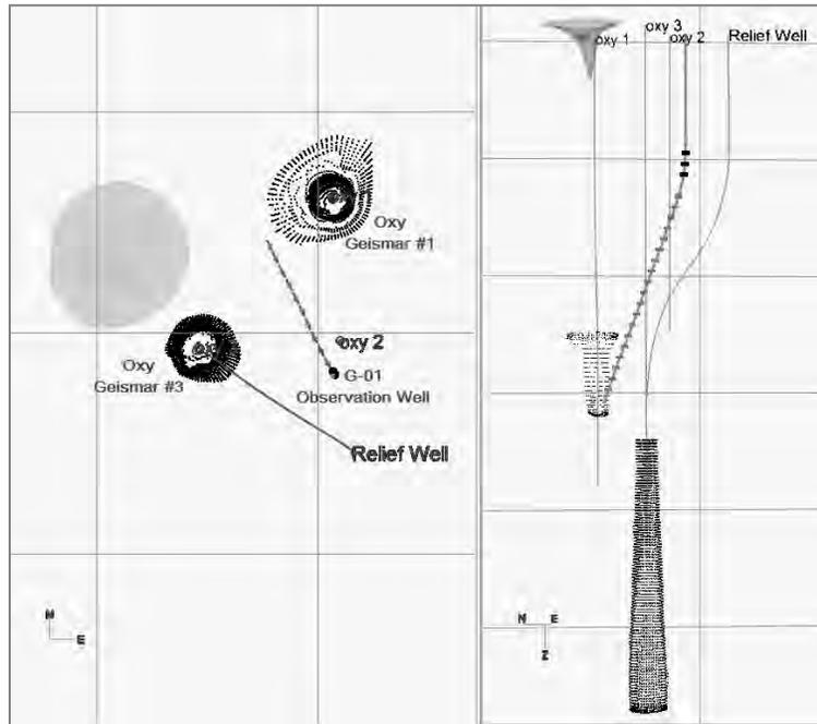
**Figure 2. G-01 well location map (left) and a vertical cross section, looking from the south (right). The Oxy Geismar 1 and 3 solution cavern outlines and the approximate location of the sinkhole are shown; grid on map and side view is 1000 feet.**
