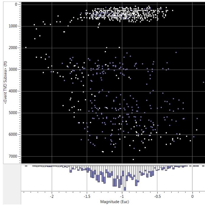
Figure 10. The distribution of Magnitude vs TVD depth for all located MEQ. The white dots and histogram bars represent MEQ in the TBC-target zone and the purple dots and histogram MEQ events located outside the TBC monitoring area.
