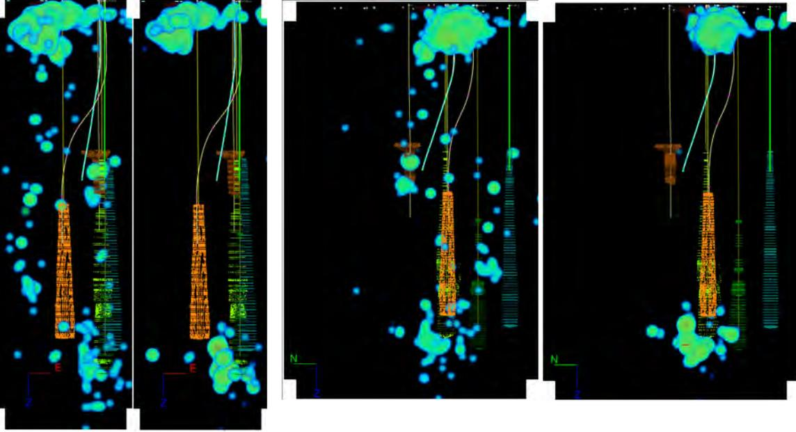
Figure 13. E-W (left plots) and N-S (right plots) cross sections of MEQ event density mapped using G-01 array scaled by number of MEQ events (left plot in the pair) and magnitude of the MEQ events (right plot in the pair).
