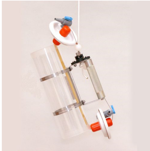
Figure 1. Vertical Van Dorn sampler
