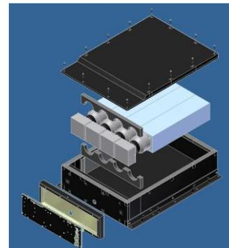
**Figure 3:** RSX-4 unit showing four detector locations. The ASPECT was equipped with 6 NaI[Tl] and 2 LaBr<sub>3</sub>:Ce scintillating detectors
