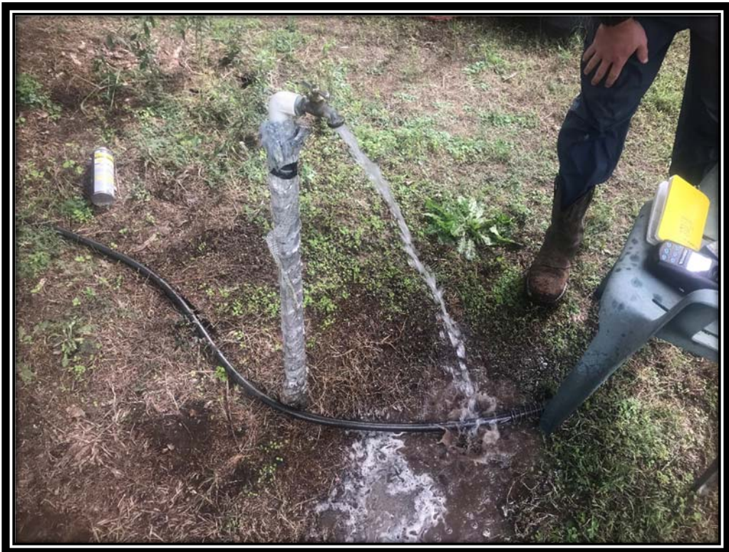
Purging and collection point
