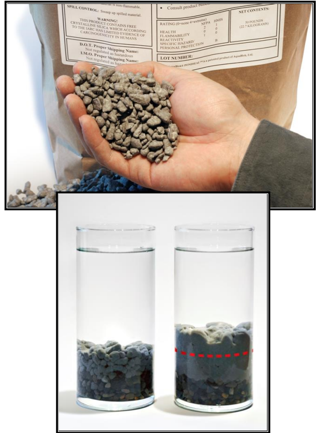
Figure 1. Configuration of stone-clay composite particle.
