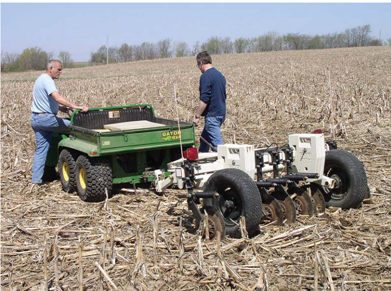
A towed electrode-array (six coulter-electrodes) soil EC_a mapping system behind a utility vehicle in a field of corn stubble.
