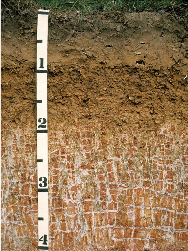
A soil in which a reticulately mottled zone with plinthite (darkest red colors) is below a depth of about 2 feet.
