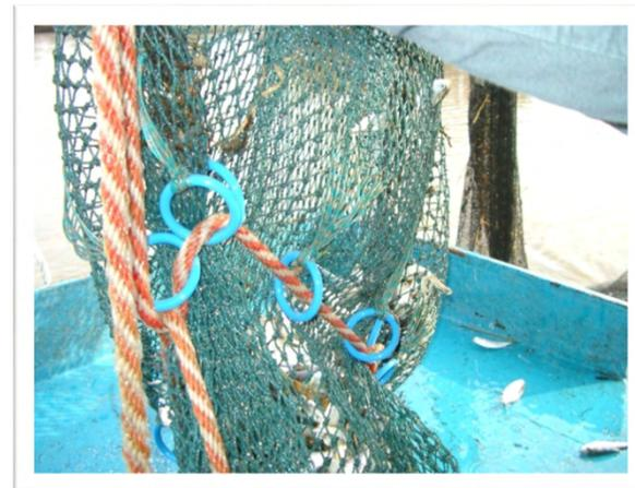
IMGP2972: The full end of the trawling net, closed by a rope looped through rings and tied with a knot that is secure, but easily released to dump the catch.
