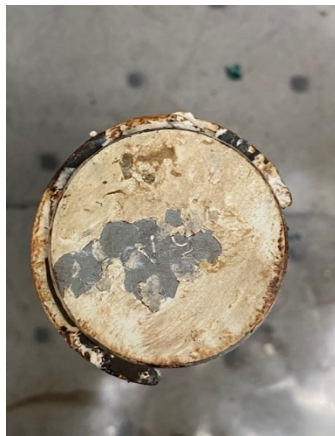
Figure 3: Pre-1990 Snap Ring without Retaining Ring
