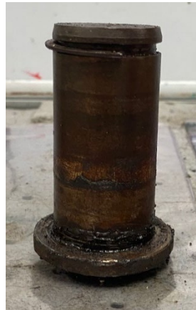
Figure 4: 1990-2010 Hinge Pin -Solid Pin with Retainer Ring
