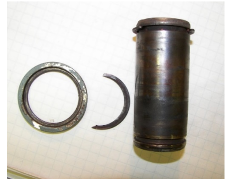
Figure 11: Broken Snap Ring.
