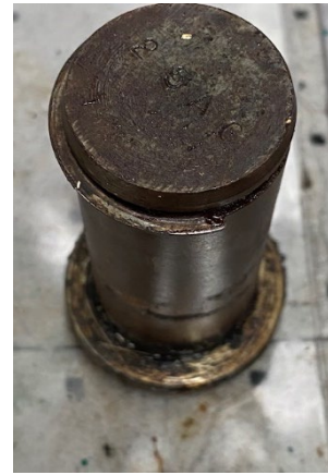
Figure 5: 1990-2010 Hinge Pin Design Solid Pin with Retainer Ring
