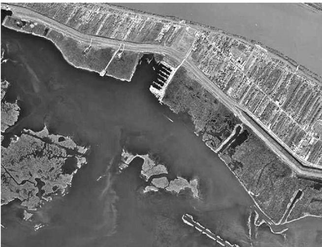
Tchefuncte River allows regular flushing at Marina Beau Chene in St. Tammany Parish. The depth of the marina basin at Bowtie Marina is shallower than the adjacent bayou, encouraging regular outflow. Tidal flow in Lake Pontchartrain sustains flushing at South Shore Harbor.
