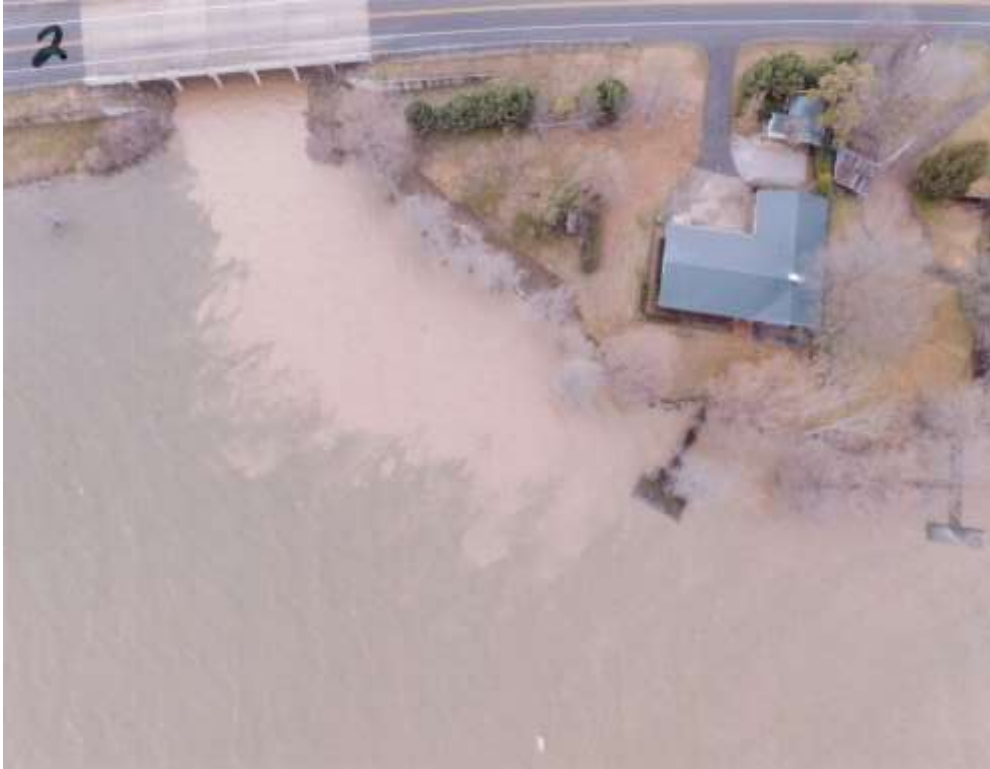
Photograph E2: Baxter Bayou outfall. Note the sediment plume.
