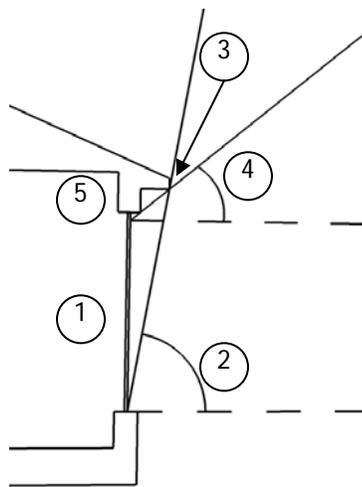
Size south overhangs using the adjacent diagram and these steps:
