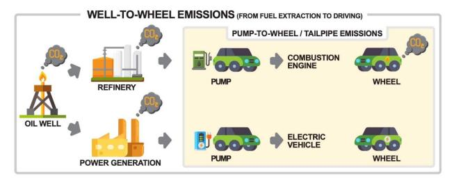
It's common for electric vehicles (and hydrogen fuel-cell vehicles) to be referred to as "Zero Emission." While electric vehicles don't have tailpipe emissions and usually have significantly lower lifetime GHG and criteria pollutant emissions than their gasoline and diesel counterparts, unless they are charged by zero-carbon electricity, they are not completely zero-carbon themselves. This is because there are still emissions related to their power generation, as shown above.
