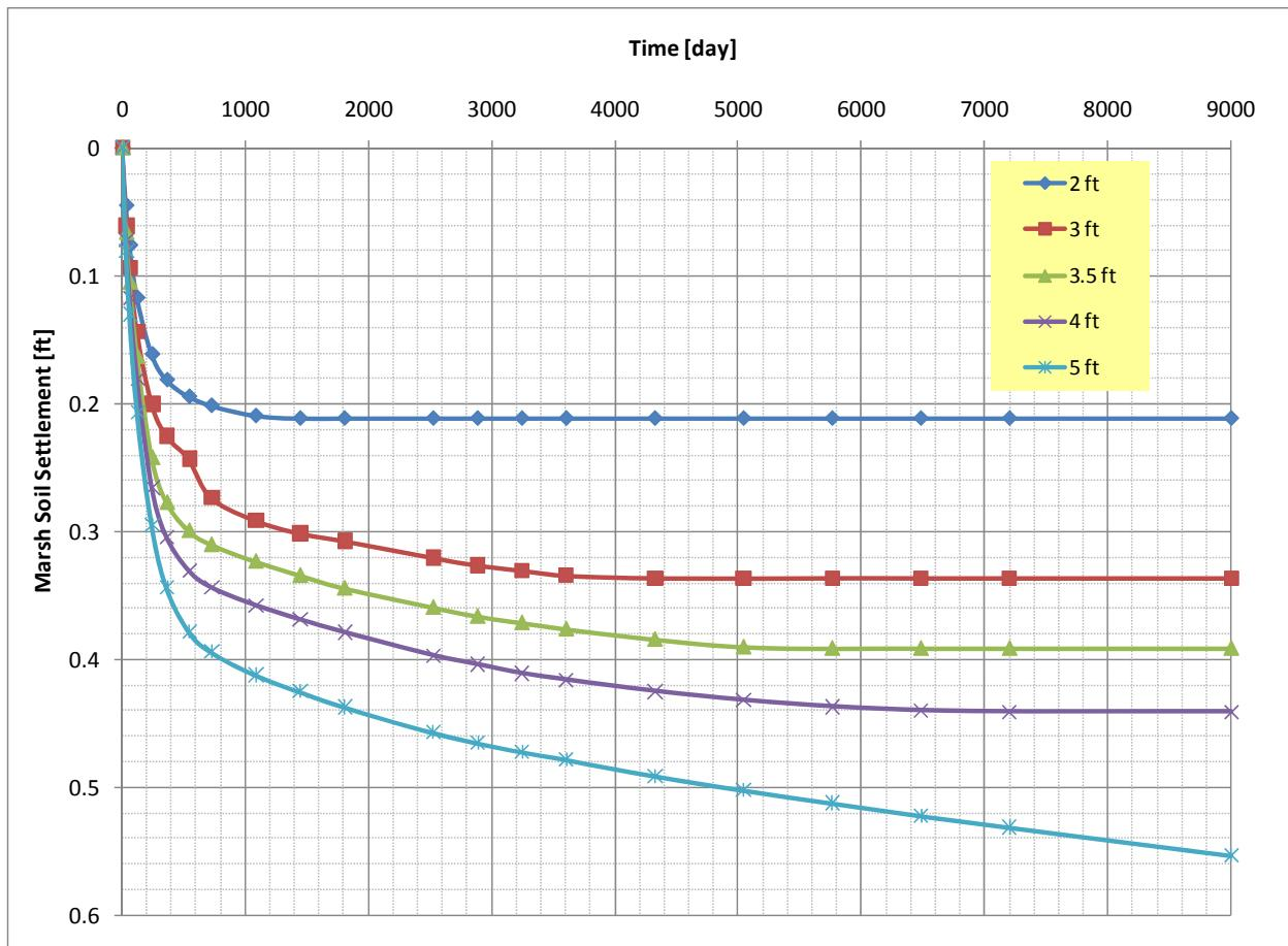
Figure 2. Case A: marsh soil settlement vs. time curves for five fill heights (2, 3, 3.5, 4, and 5 ft above the marsh soil).
