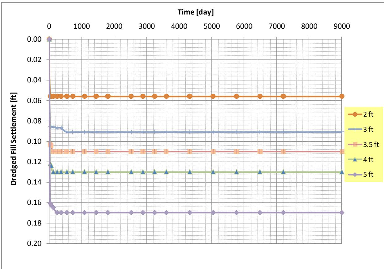
Figure 3. Case A: fill settlement vs. time curves for five fill heights (2, 3, 3.5, 4, and 5 ft above the marsh soil).
