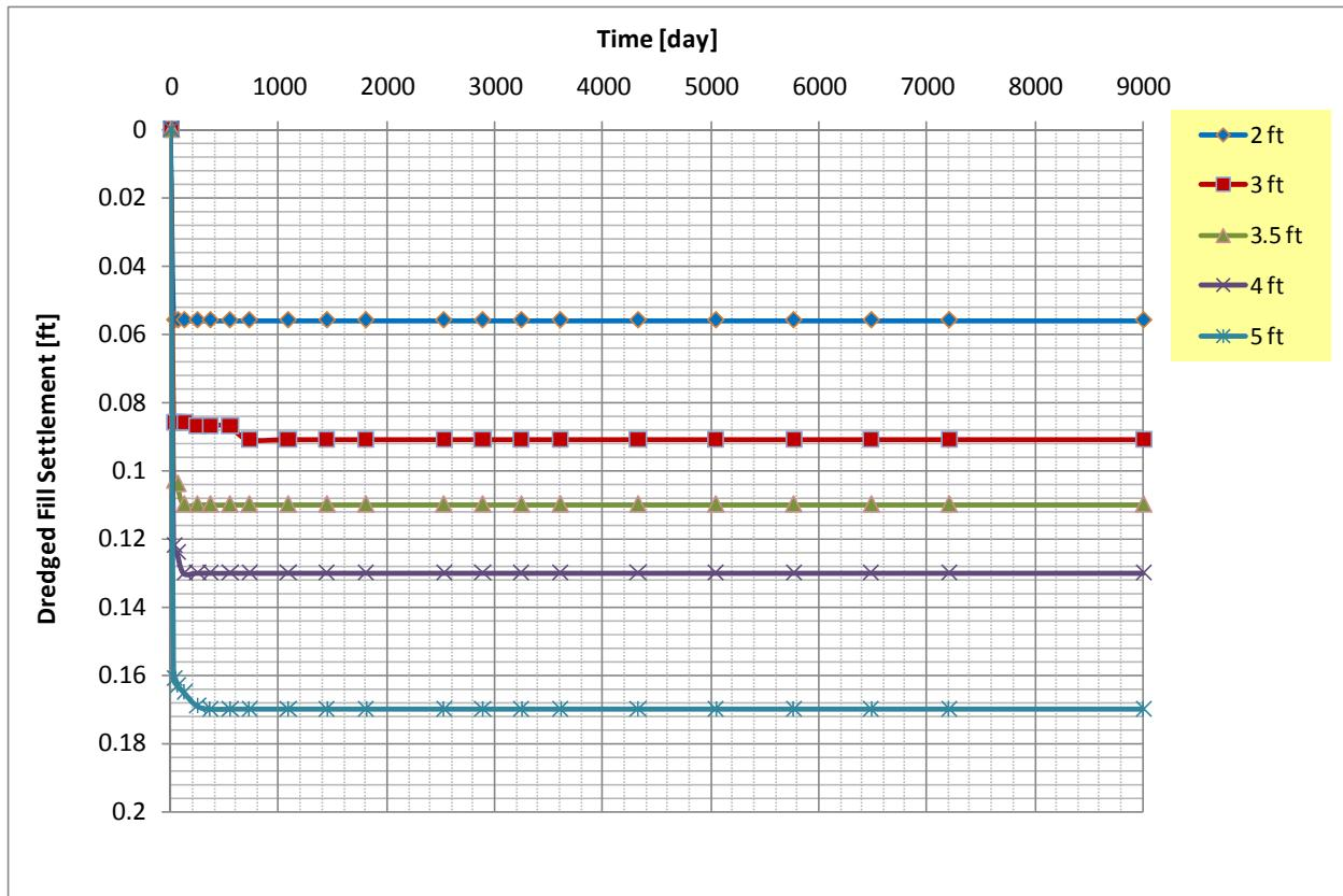
Figure 6. Case B: fill settlement vs. time curves for five fill heights (2, 3, 3.5, 4, and 5 ft above the marsh soil).
