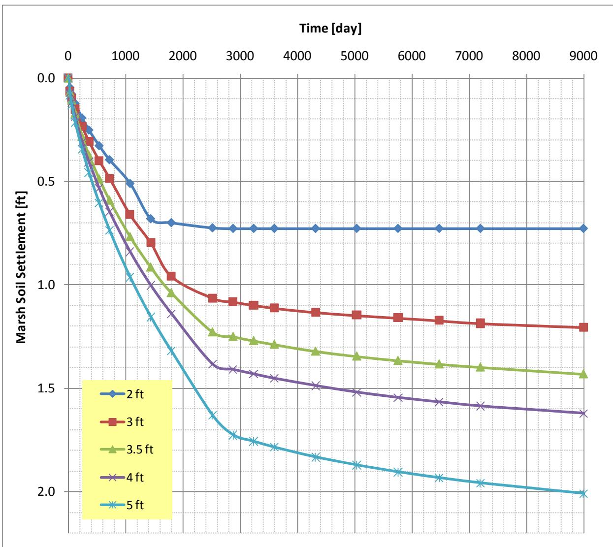
Figure 5. Case B: marsh soil settlement vs. time curves for five fill heights (2, 3, 3.5, 4, and 5 ft above the marsh soil).
