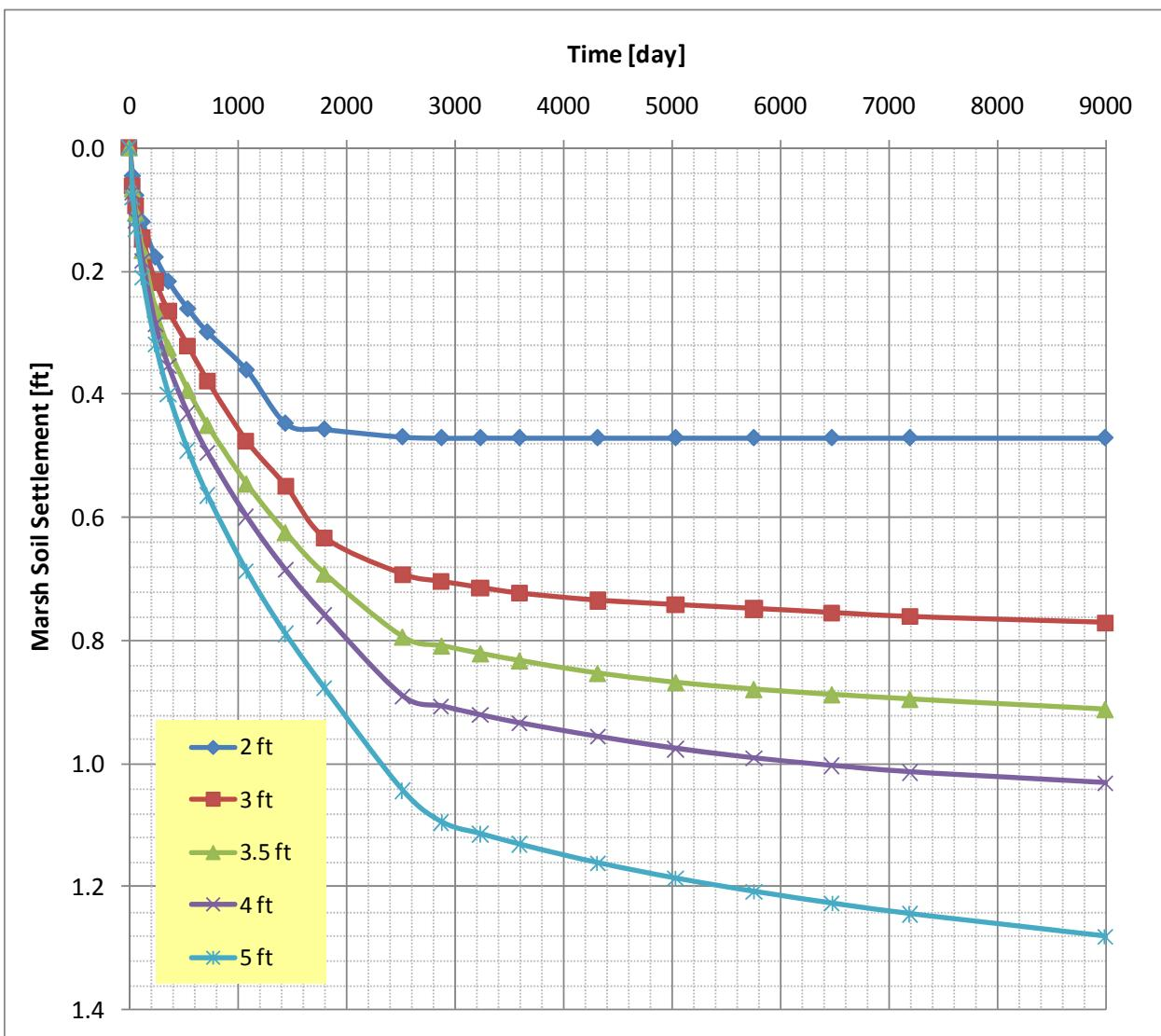
Figure 8. Case C: marsh soil settlement vs. time curves for five fill heights (2, 3, 3.5, 4, and 5 ft above the marsh soil).
