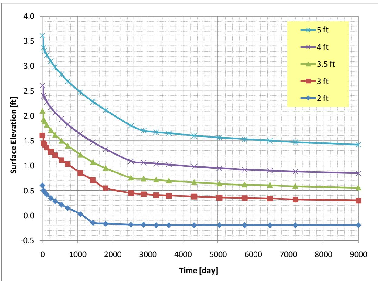
Figure 4. Case B: surface elevation vs. time curves for five initial fill heights (2, 3, 3.5, 4, and 5 ft above the marsh surface).
