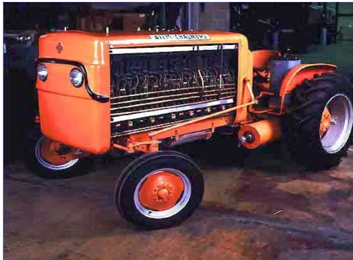
Figure 2 - Allis Chalmers Alkaline Fuel Cell Powered Tractor (Courtesy of the Smithsonian Institute)
