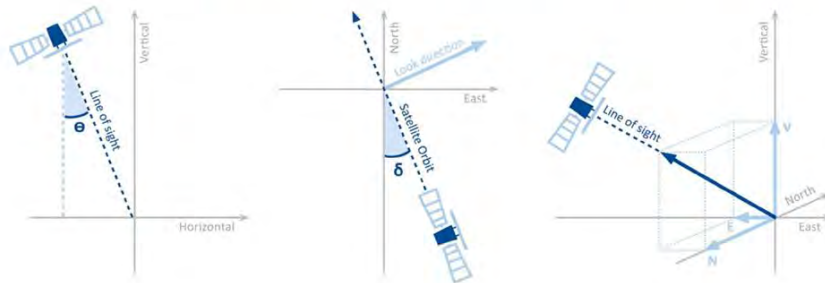
Figure 29: Example of metadata associated to the SqueeSAR measurements. LOS angles and versors can be used to transform a 3-D measurement ( D_{VERT} , D_{EW} and D_{NS} ) onto a LOS measurement ( D_{LO} ).
