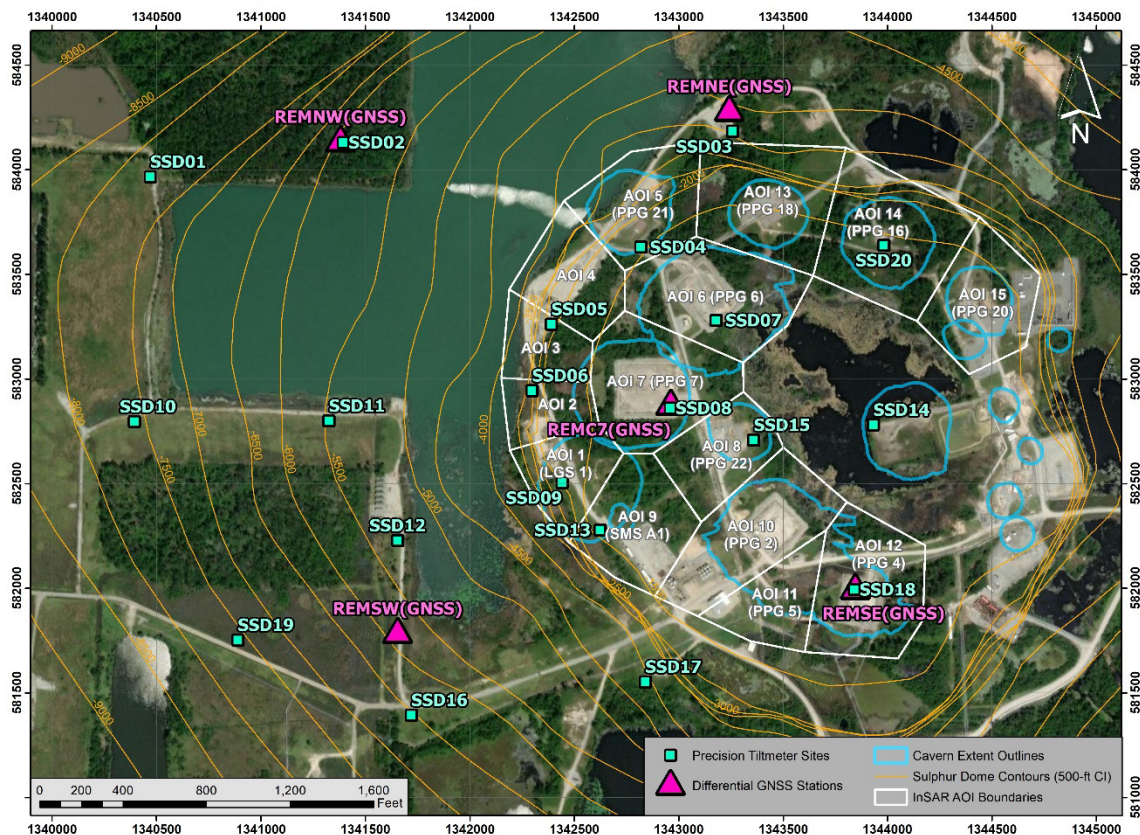
Figure 1. Map of the tiltmeter and GNSS network installed at Sulphur Mines dome. The cyan squares indicate the tiltmeter site locations. The GNSS stations are shown by pink triangles. The InSAR AOI boundaries are shown for reference. The surface projection of the various salt caverns is indicated by blue lines. The salt dome contours are in light orange. The backdrop is an aerial photograph of the Sulphur Mines salt dome.
