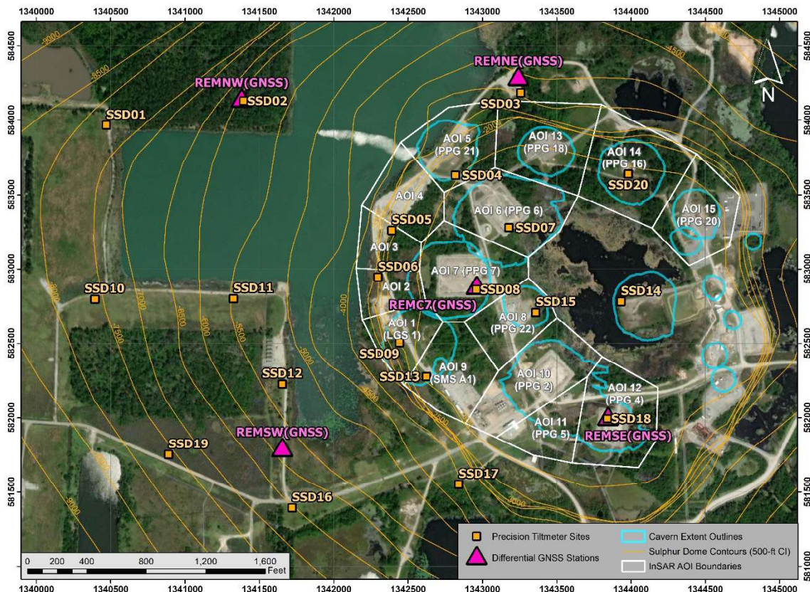
Figure 1. Map of the tiltmeter and GNSS network installed at Sulphur Mines dome. The orange squares indicate the tiltmeter site locations. The GNSS stations are shown by pink triangles. The InSAR AOI boundaries are shown for reference. The surface projection of the various salt caverns is indicated by cyan lines. The salt dome contours are in light orange. The backdrop is an aerial photograph of the Sulphur Mines salt dome.
