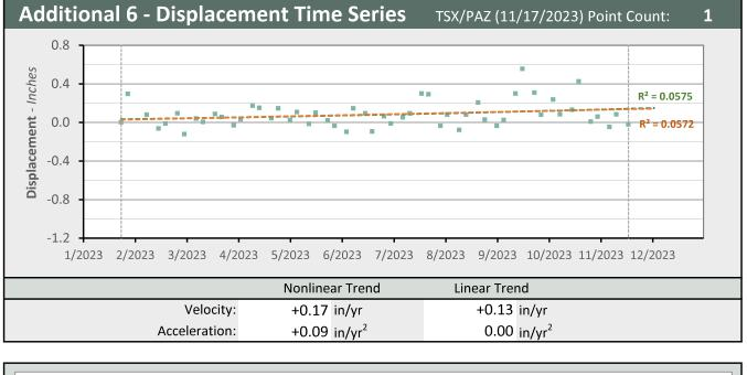
Nonlinear Trend Line LOS Displacement Measurement
