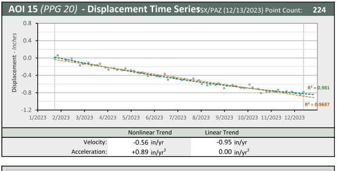
Nonlinear Trend Line Linear Trend Line LOS Displacement Measurement (Quadratic Regression)
