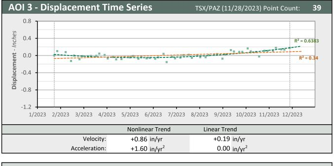
Nonlinear Trend Line LOS Displacement Measurement
