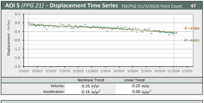
Nonlinear Trend Line LOS Displacement Measurement
