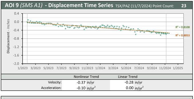
Nonlinear Trend Line LOS Displacement Measurement
