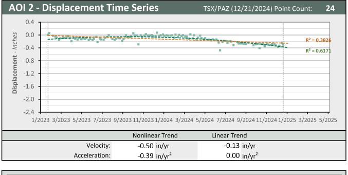
LOS Displacement Measurement Nonlinear Trend Line Linear (Quadratic Regression)
