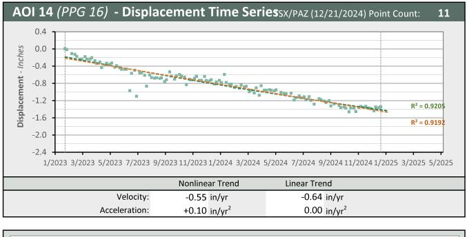
LOS Displacement Measurement ---- Nonlinear Trend Line Linear Trend Line (Quadratic Regression) Linear Regression)
