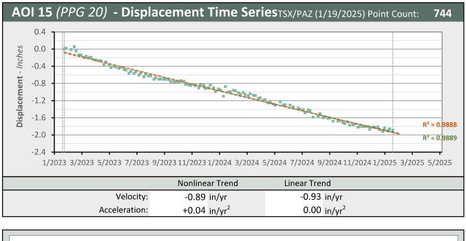
LOS Displacement Measurement ---- Nonlinear Trend Line (Quadratic Regression) Linear Trend Line (Linear Regression)
