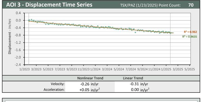
LOS Displacement Measurement Nonlinear Trend Line Linear Trend Line (Quadratic Regression)
