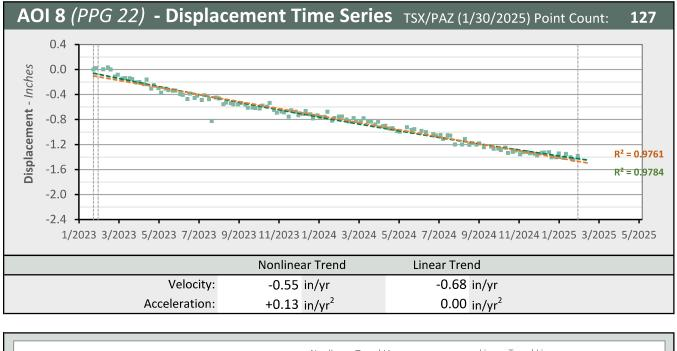
LOS Displacement Measurement ---- Nonlinear Trend Line Linear Trend Line (Quadratic Regression) (Linear Regression)
