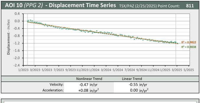
LOS Displacement Measurement Nonlinear Trend Line Linear Trend Line (Quadratic Regression)
