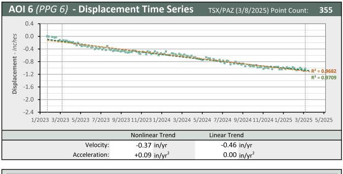
Nonlinear Trend Line Linear Trend Line LOS Displacement Measurement \_ (Quadratic Regression) (Linear Regression)
