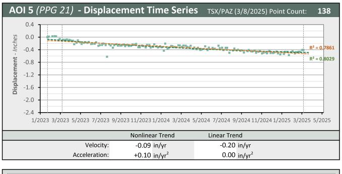
Nonlinear Trend Line Linear Trend Line LOS Displacement Measurement \_ -----(Quadratic Regression) (Linear Regression)
