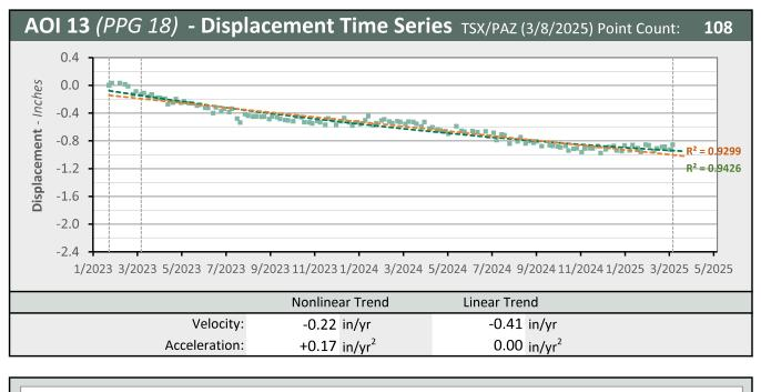
Nonlinear Trend Line LOS Displacement Measurement \_ (Quadratic Regression)
