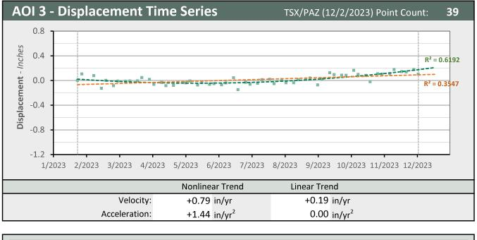
Nonlinear Trend Line LOS Displacement Measurement
