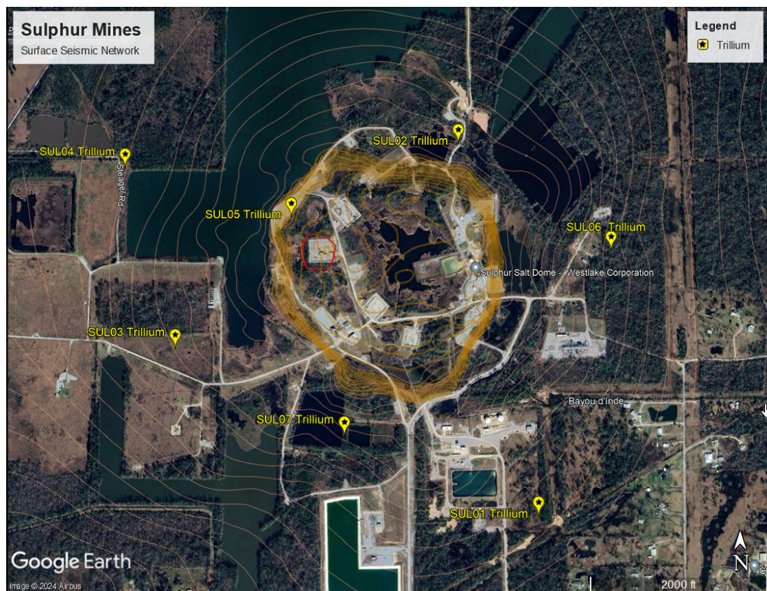
Figure 13. Google Earth map image showing the location of the six broadband seismic (Trillium Compact Sensors, yellow symbols and labels) stations near and at the Sulphur Mines Salt Dome. The contours are the salt and cap rock elevations, the red circle is the general outline of Cavern 7.
