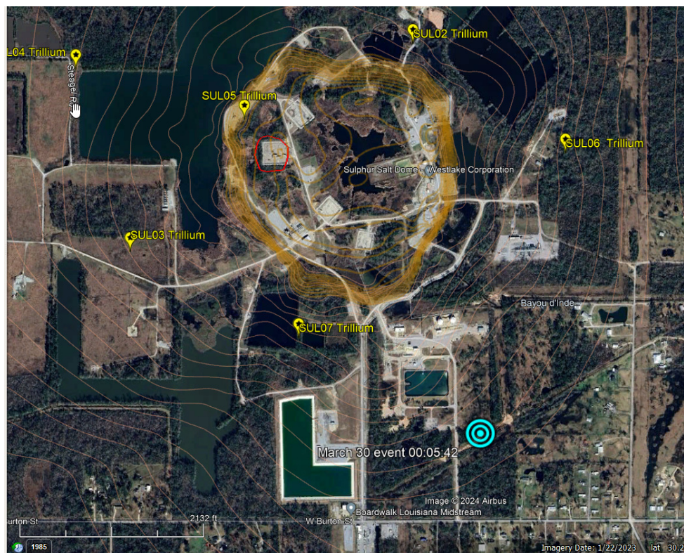
Figure 1. Google Earth image of Sulphur Mines salt dome area. The March 30, 2024 event location is shown by a cyan dot. The seismic station locations are shown by yellow symbols.
