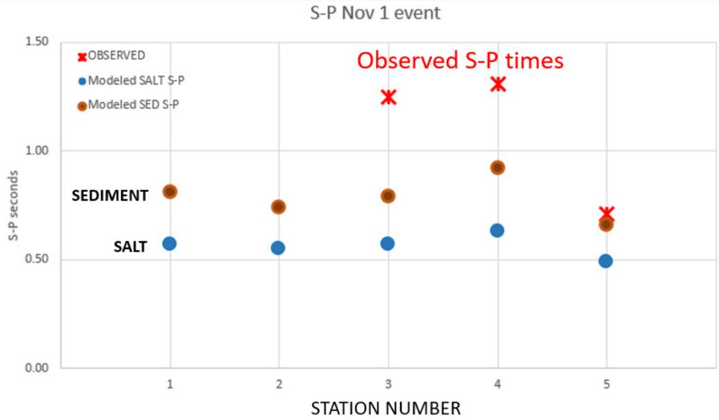
Figure 5. A graph of the observed S-P times on the broadband station for the seismic detection on November 1. The plot also shows the modeled S-P times for an event either on the salt dome (blue dots) or sediments near Cavern 7 (brown dots) at 2500 ft depth. The red stars are the observed S-P times at Station 3, 4 and 5 which are not compatible with an event near Cavern 7.
