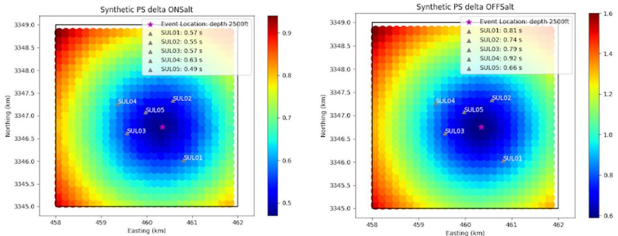
Figure 4. Modeled S-wave minus P-wave travel times for a theoretical event occurring at Cavern 7 at 2500 ft depth. The left plot shows travel times for an event within the salt dome (“on salt”) and the right plot shows the travel times for events outside the salt dome (“off salt”). The S-P time for each station is listed on each plot.
