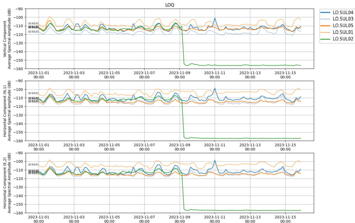
Figure 2. Average spectral amplitudes in decibels on the five broadband sensor from November 1-15, 2023. The upper plot is the vertical component, the middle and lower plots are the horizontal component (middle is north-south and lower plot is east-west component).
