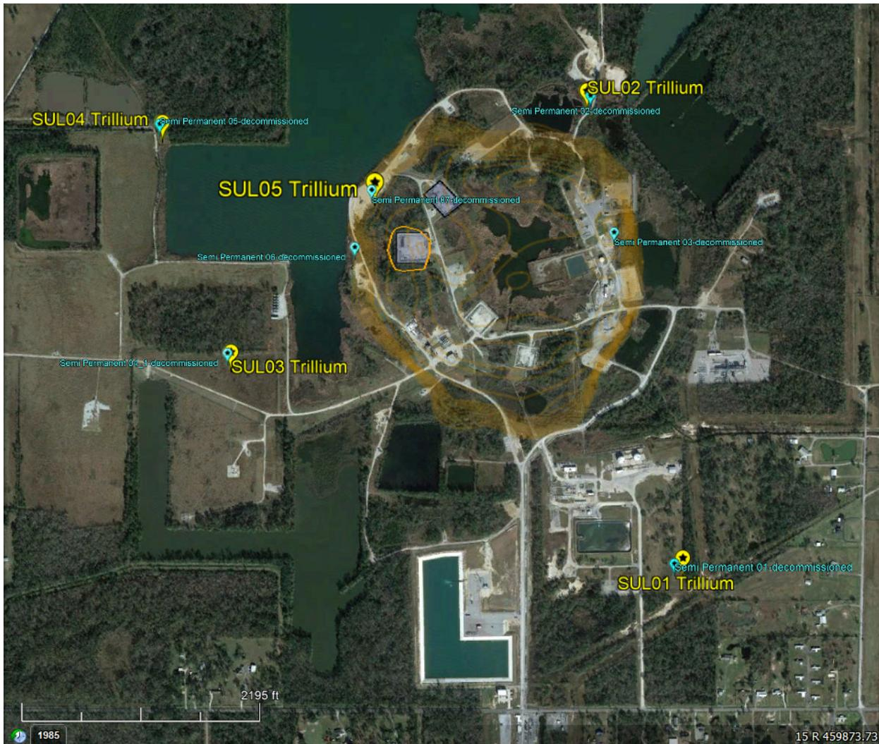
Figure 1. Google map image showing the location of the decommissioned semi-permanent (4.5 Hz sensors, aqua symbols and labels) and broadband seismic (Trillium Compact Sensors, with yellow symbols and labels) stations near and at the Sulphur Mines Salt Dome.
