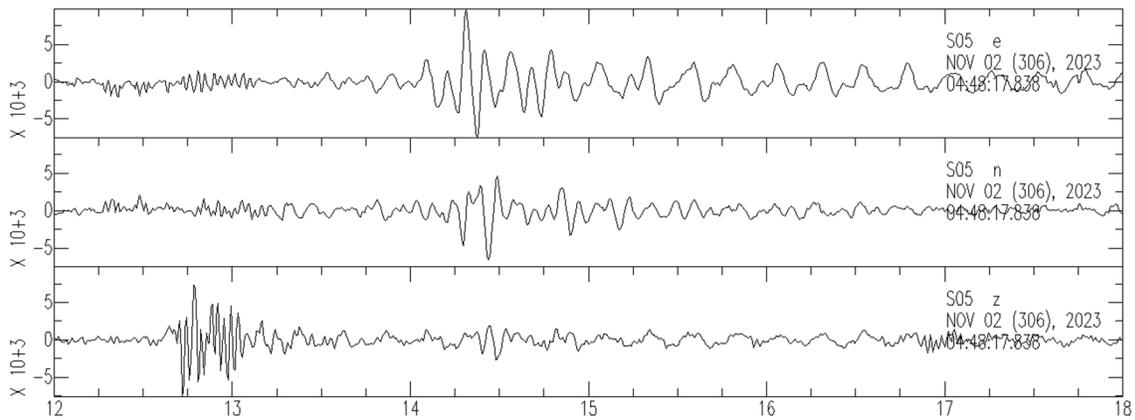
Figure 3. Waveforms recorded on the 4.5 Hz geophone at semi-permanent station 5 on November 1 11:48 (UTC time November 2 04:48). The upper plot is the east component, the middle plot the north component the lower plot is the vertical component. The scale on the bottom is seconds.
