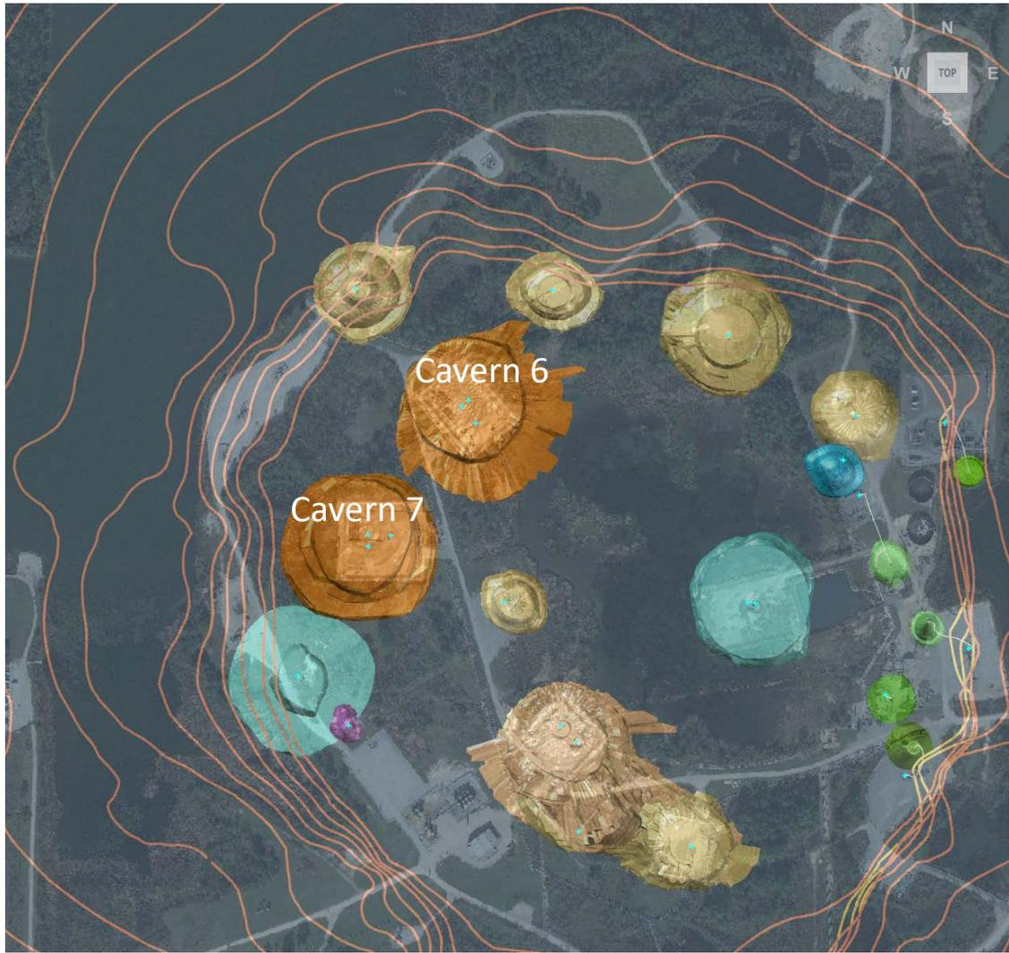
Figure 4 – Plan View Color Coded Image of All Salt Caverns in Sulphur Mines Dome
