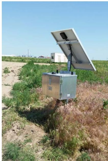
Figure 44 – Example of a JDS Pole-Mounted Seismic Station
