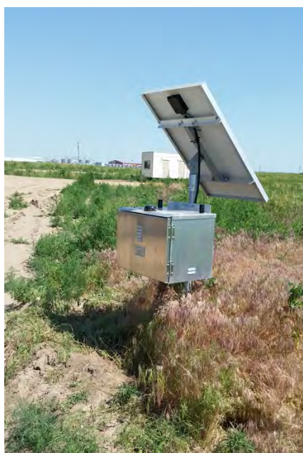
Figure 2. An example of a JDS pole-mounted seismic station.
