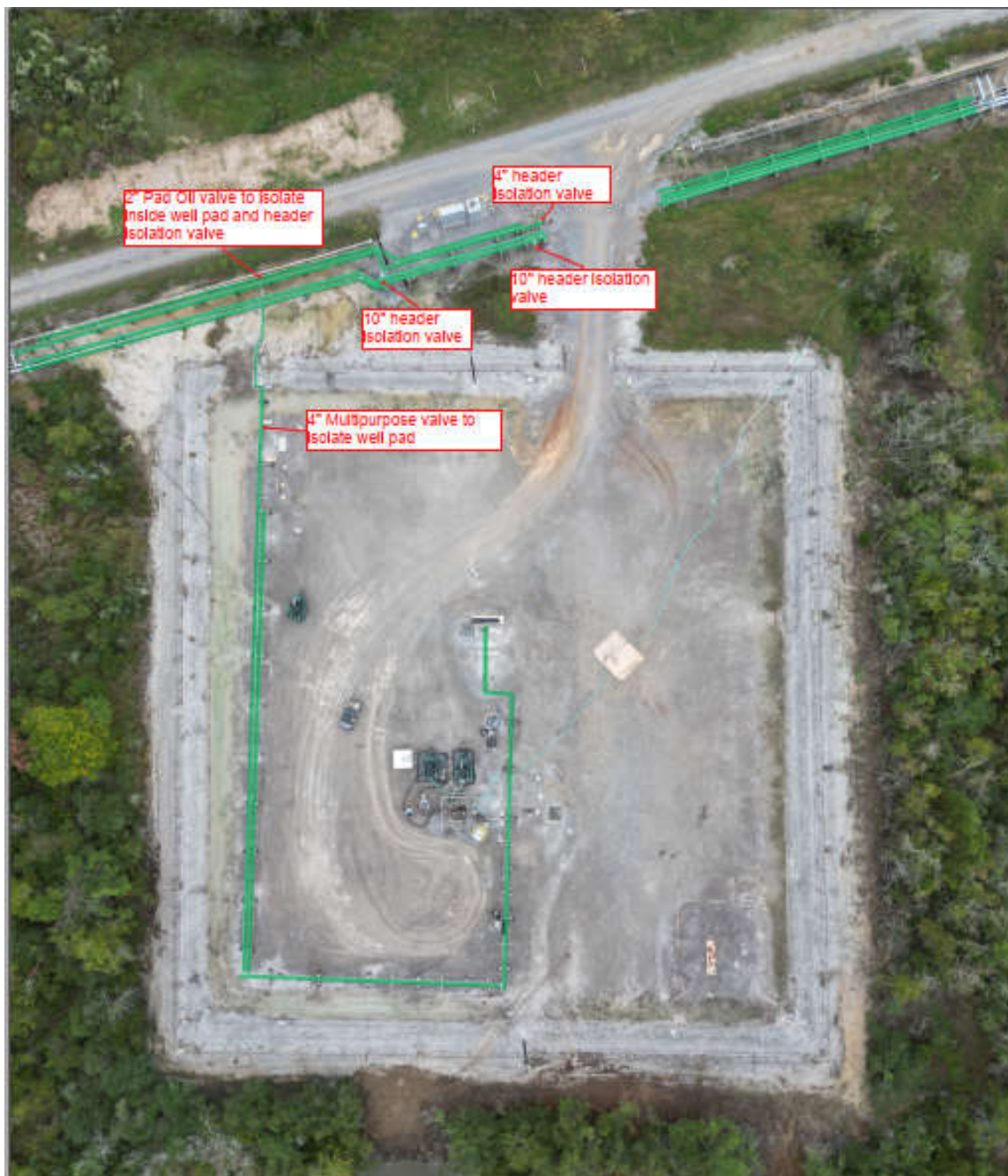
Figure 3 – No. 7 Brine Well Pad Isolation and Demolition Aerial Photograph
