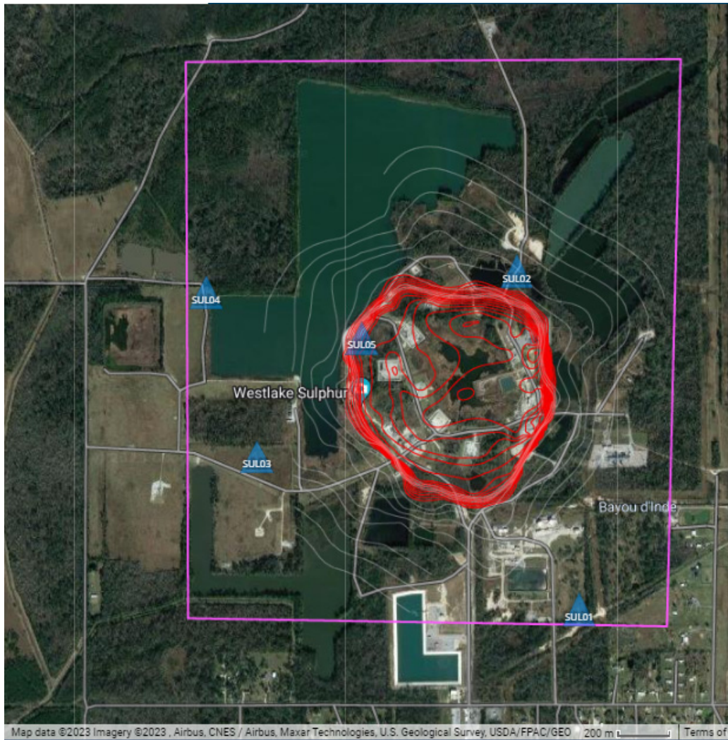
Figure 1. Map showing the location of Nanometrics Seismic Array stations (blue triangles) at Sulphur Mines dome. The gray lines show the contour lines of the salt dome and red lines show the cap rock contour lines. The purple line is the outline of the seismic monitoring AOI.
