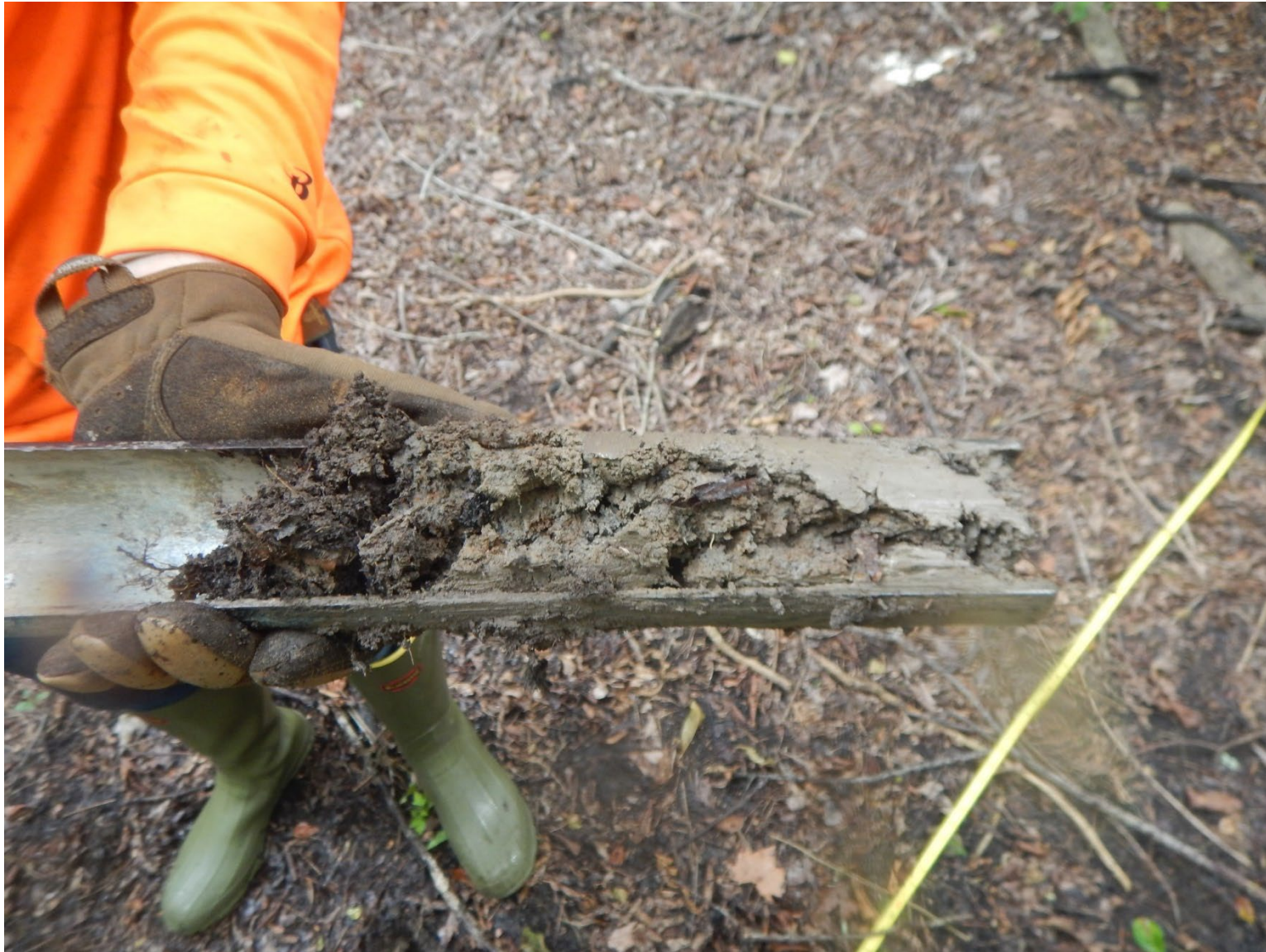
Figure 23. Zone IV soil mucky clay surface layer.
