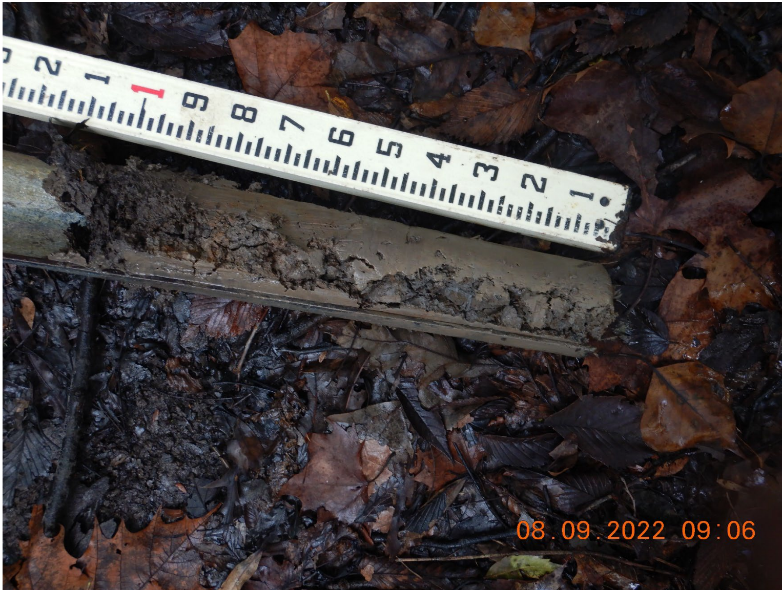
Figure 21. Zone III soil – mucky clay surface layer
