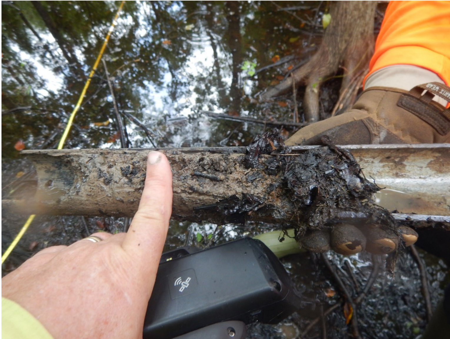
Figure 15. Zone II soil muck layer.
