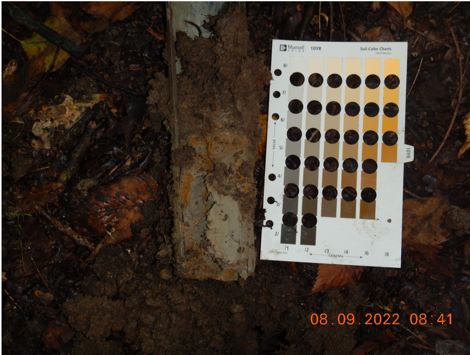
Figure 25. Zone 5 soil – low organic surface layer but wetland indicators at depth.
