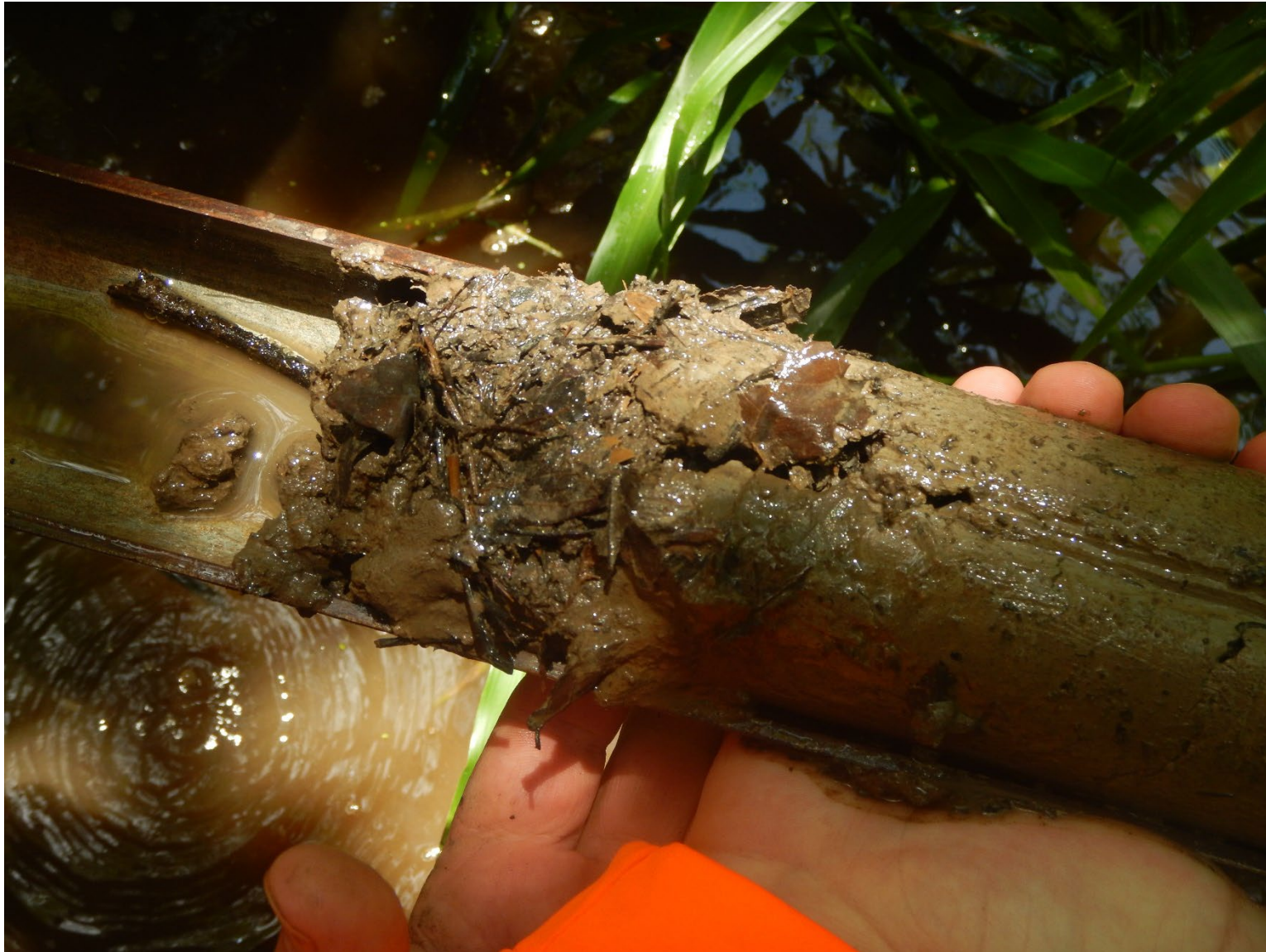
Figure 17. Zone II muck layer evident
