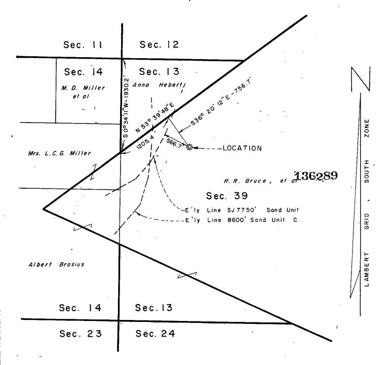
WELL LOCATION: From the Northwest corner of Section 13, T-10-S, R-3-W, go S 0°34'11"W 1930.2 feet to the westerly line of Section 39, T-10-S, R-3-W; thence, N 53°39'48"E along the westerly line of said Section 39, 1205.4 feet; thence, at right angles S 36°20'12"E-756.7 feet to location in said Section 39, T-10-S, R-3-W, Jefferson Davis Parish, Louisiana.
