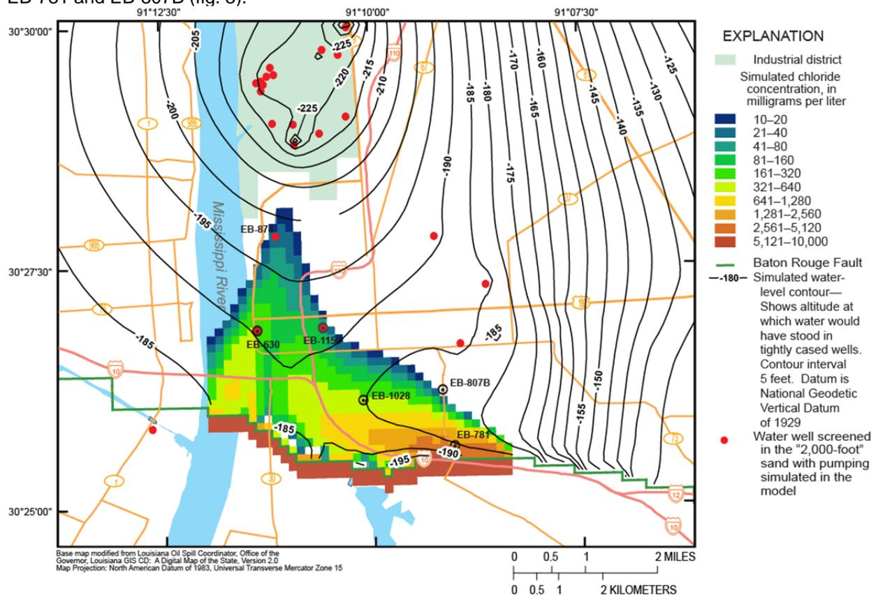
**Figure 3. Simulated 2012 water levels and chloride concentrations at the base of the “2,000-foot” sand of the Baton Rouge area in the detailed model area in southeastern Louisiana.**
