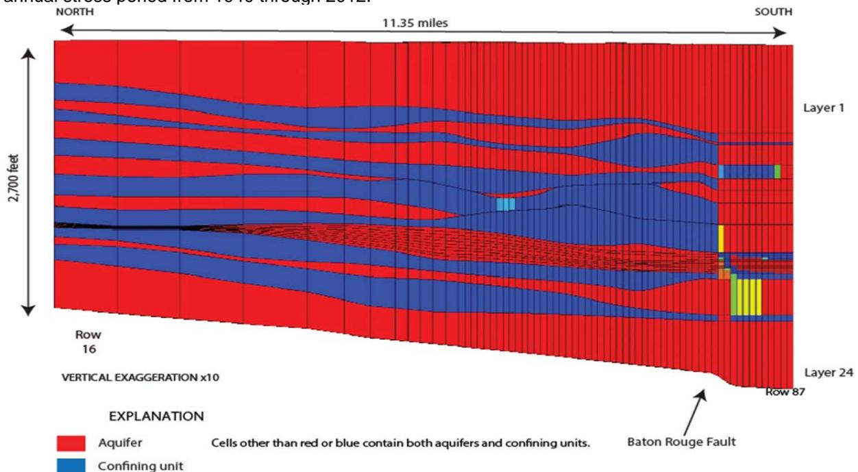
**Figure 2. North-South vertical section along column 24 from row 16 to row 87 showing aquifer and confining layers.**
