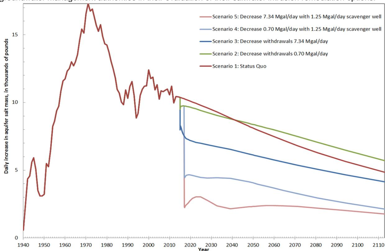
**Figure 4. Simulated changes in salt mass in the “2,000-foot” sand of the Baton Rouge area north of the Baton Rouge Fault, 1940-2012, and predicted changes in salt mass during 5 hypothetical pumping scenarios, 2013-2112.**
