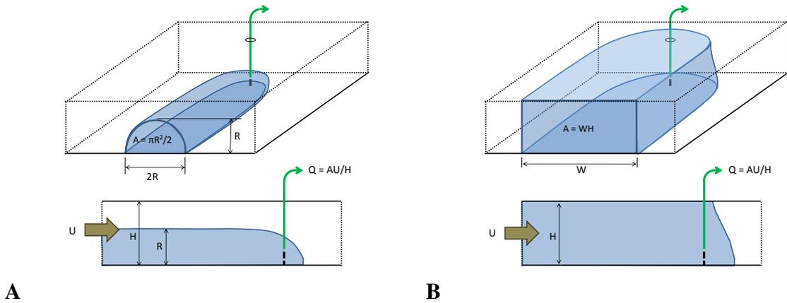
Figure 32: Conceptual sketches of the capture zones for a partially penetrating well of small discharge (A) and large discharge (B).
