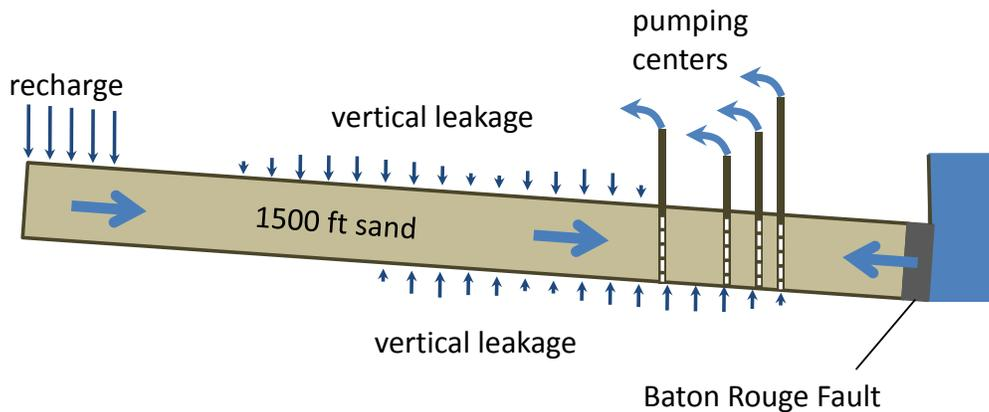
Figure 16: Conceptual sketch of flow in the 1,500-Foot sand. North-to-south section through the aquifer (*not to scale*).
