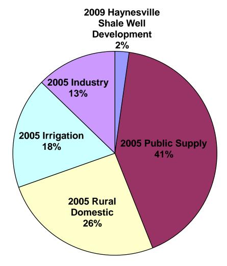
Note: In 2009, 64% of oil and gas wells reporting water usage in their work history used water wells in the Wilcox aquifer. There were 292 gas wells completed in 2009. The average water use of a Haynesville Shale Wilcox water well is 818,340 gallons per well. Net wells using water from the Wilcox aquifer: 64% x 292 = 187 wells. Net Water Use: (187 wells x 818,340 gallons of water per well)/365 days ≈ 419,000 gallons/day
