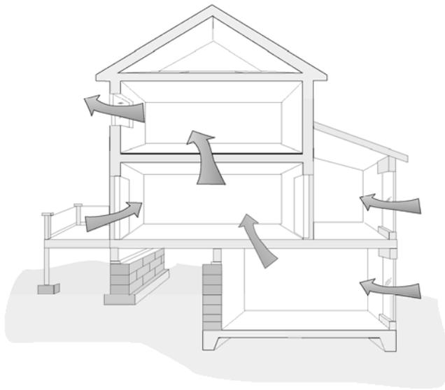
As the interior air heats up it rises to the higher parts of the structure and escapes creating suction. The suction pulls in cooler (lower) air from outside. The structure behaves like a chimney cooling and aerating the house. The taller the structure, the stronger the force. This effect is why most old plantation homes have such high ceilings and double hung windows.
