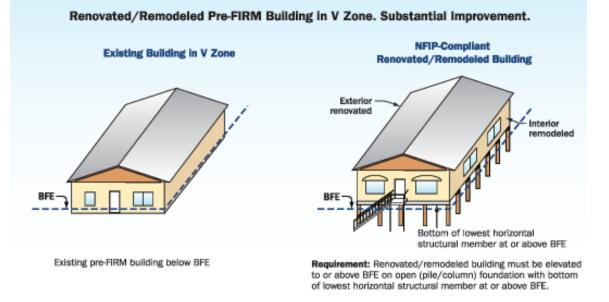
**Figure 6-4.** When an owner makes substantial improvements or additions to an existing home, the LSUCC mandates that the entire structure meet IRC standards. This may require that an entire structure be raised above BFE (From FEMA. 2005. *Home Builder's Guide to Coastal Construction, Fact Sheet No. 30, FEMA 499-CD*).
