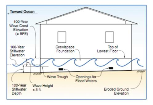
**Figure 2-3.** NFIP requires that structures located in A Zones be elevated at or above BFE. As in V Zones, elevation should include freeboard to decrease risk of damage (From FEMA. 2000. *Coastal Construction Manual, FEMA 55*).
