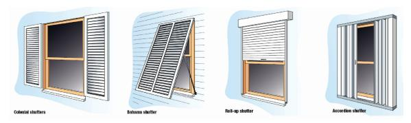
**Figure 6-12.** Different types of shutters used for window protection (From FEMA. 2005. *Home Builder's Guide to Coastal Construction, Fact Sheet No. 26, FEMA 499-CD*).
