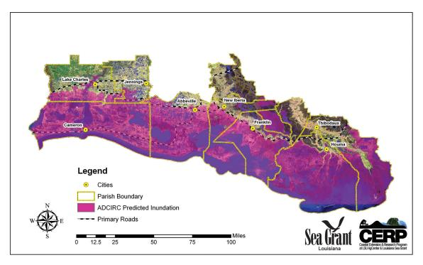
**Figure 1-8.** ADCIRC simulation of predicted storm surge from Hurricane Rita — Note that the predicted extent of storm surge simulated by the ADCIRC model nearly mirrors the observed storm surge, which is shown in Figure 1-9 for comparison (Image courtesy of M. Wolcott, based on ADCIRC modeling by H. Mashriqui).
