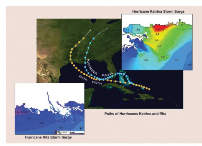
Fig. 3. A composite figure showing paths of Hurricanes Katrina and Rita, surge levels [in meters, as estimated by the ADCIRC model (67)], areas flooded, sites of levee failures, and wetland loss due to the hurricane.
