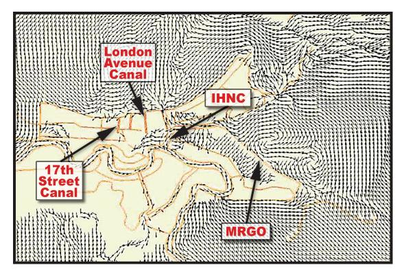
**Figure 1-10.** ADCIRC simulation of water circulation generated by Hurricane Katrina around New Orleans and over the tops of levees at the onset of flooding -- Note that the triangular "funnel" opening to the east includes flows along and across the levees and floodwalls shown in pink (From Ivor LI. Van Heerden *et al.* Team Louisiana. 2006. *The Failure of the New Orleans Levee System during Hurricane Katrina*).
