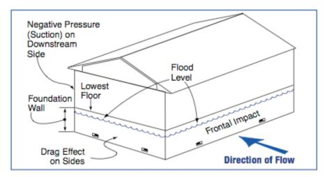
**Figure 6-8.** Hydrodynamic loads on buildings (From FEMA. 2000. *Coastal Construction Manual, FEMA 55*).
