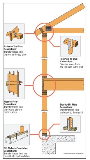
Figure 6-10. Key components of continuous load path connections (Courtesy of Simpson Strong-Tie).
