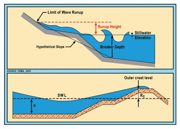
**Figure 1-14**. Hurricane-generated waves ride on top of the surge and turn levees and inland bluffs into beaches that can be eroded by the high-velocity flows that occur when waves break and water rushes uphill beyond the surge elevation. Overtopping raises the potential for erosion on the back side of levees (Adapted from FEMA. 2003. *Guidelines and Specifications for Flood Hazard Mapping Partners*).
