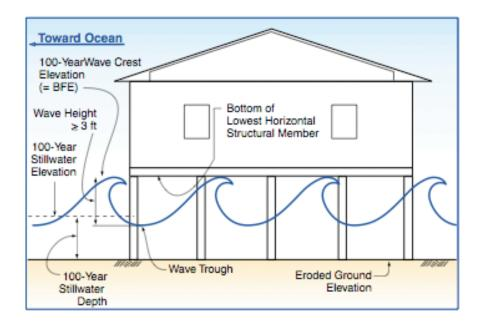
**Figure 2-2.** NFIP requires that structures located in V Zones be elevated above the BFE and built on an open foundation. Ideally, elevation should include freeboard (From FEMA. 2000. *Coastal Construction Manual, FEMA 55*).
