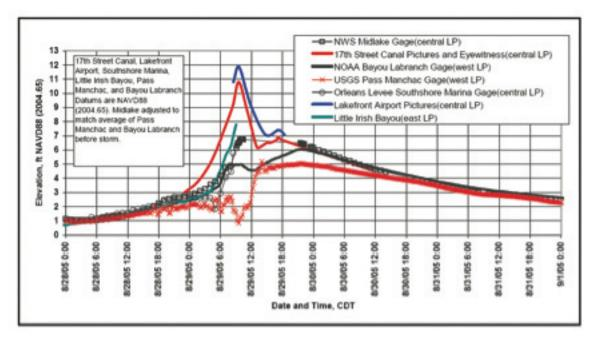
**Figure 1-13.** Storm surge on the south shore of Lake Pontchartrain (on the north side of New Orleans) reconstructed from partial gage data and from time-stamped photographs (From Interagency Performance Evaluation Taskforce. 2007. *Evaluation of the New Orleans and Southeast Louisiana Hurricane Protection System.*
