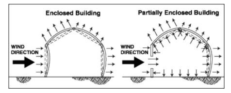
**Figure 6-1.** Effects of Wind Loads on a Structure – It is important to maintain the building envelope to avoid the types of internal wind loads show in the house on the right (From FEMA. 2000. *Coastal Construction Manual, FEMA 55*).
