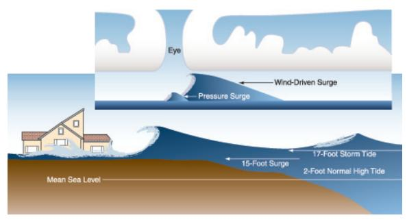
**Figure 1-3.** Storm surge as a hurricane moves ashore (From FEMA. 2006. *Recommended Residential Construction on the Gulf Coast, FEMA 550*).
