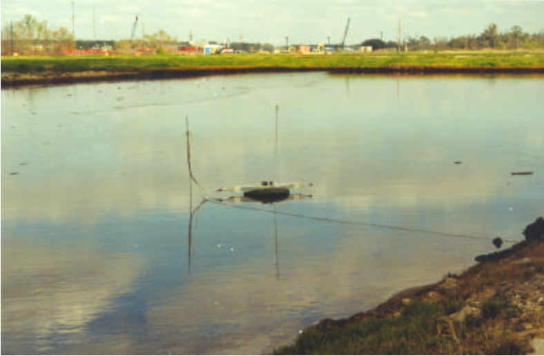
Figure 3-2 C. Placement of a flux chamber in a cell at Bateman Island
