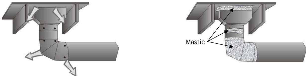
Figure 8-10 Sealing Leaky Boots
