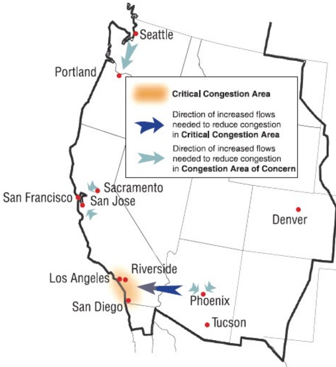
Figure 2. One Critical Congestion Area and Three Congestion Areas of Concern in the Western Interconnection
