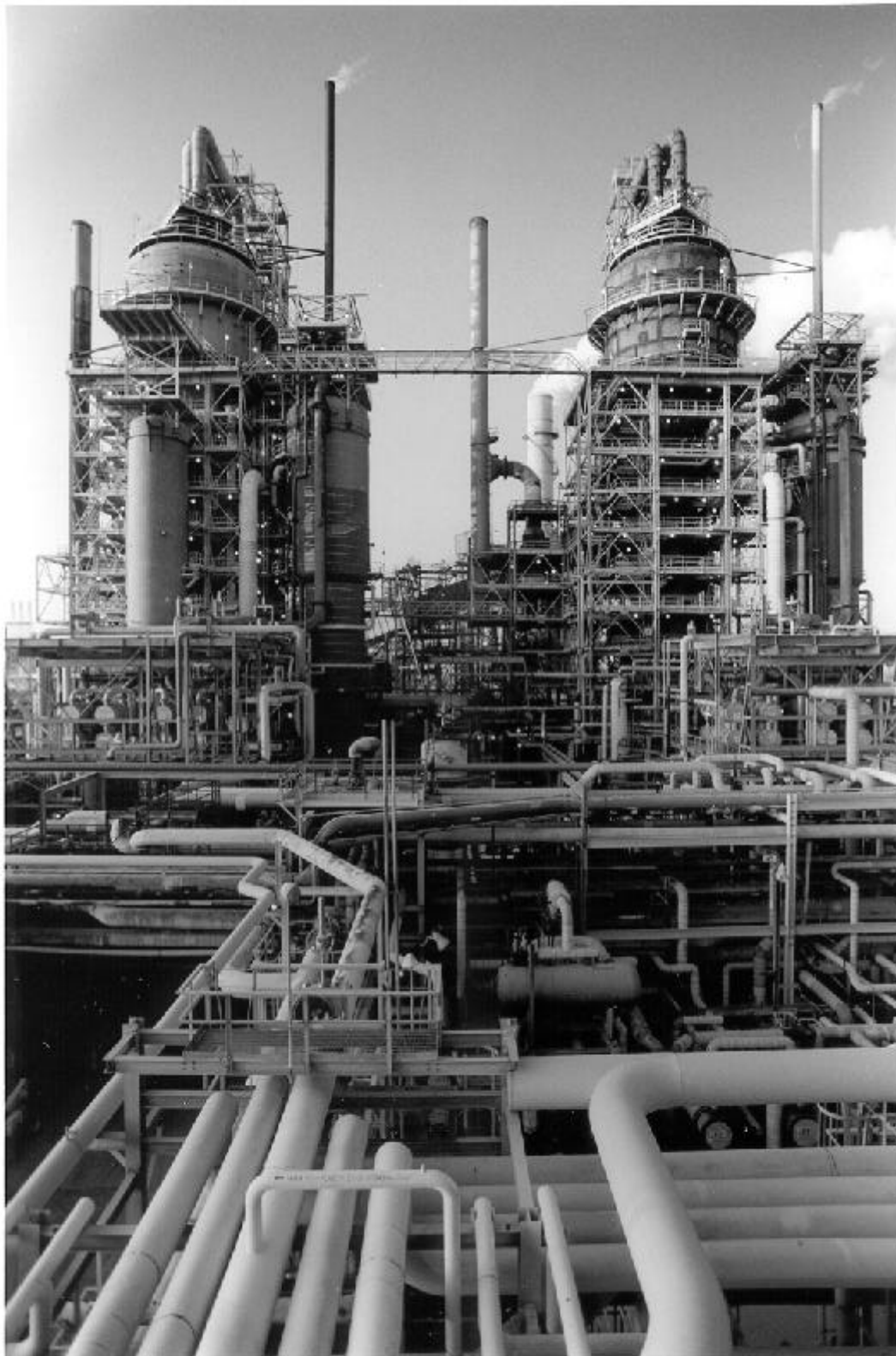
Catalytic-cracking technology invented at Exxon Baton Rouge in 1942, helped win WWII. It remains an industry standard. Photo courtesy Exxon Public Affairs.
